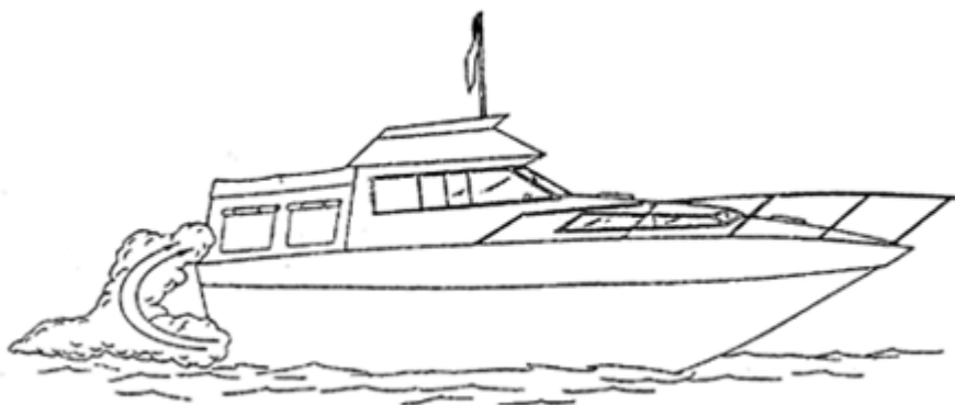
Figure A.7 — Inefficient trim angles
