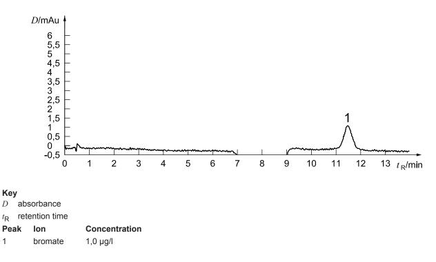
Figure 3 — Example of a chromatogram of a standard solution conforming to this International Standard
