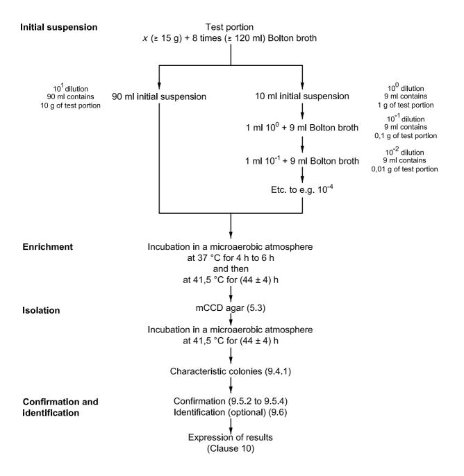
Figure A.1 — Diagram of procedure
