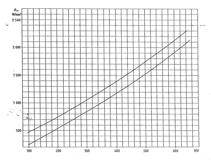
NOTE — The tensile strength values obtained by conversion can under no circumstances replace the values specified in product standards and their use does not obviate the need to carry out the tensile test.
