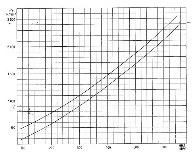
NOTE — The tensile strength values obtained by conversion can under no circumstances replace the values specified in product standards and their use does not obviate the need to carry out the tensile test.
