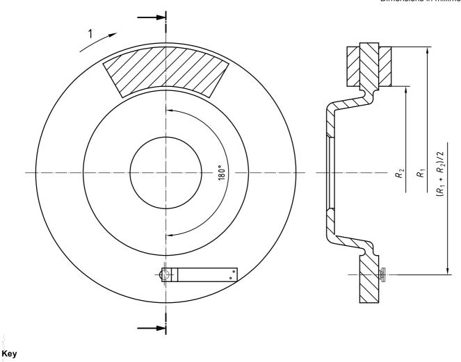
Figure B.6 — Thermocouple position — Disc brake
