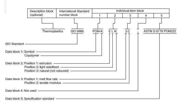
Specification: ISO 9988-POM-K,ELN,2-2,,ASTM D 6778 POM222
