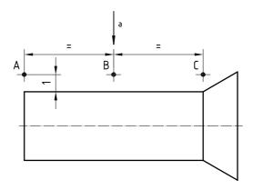
A, B and C are the measurement positions.
