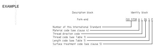
Where the following codes are applied for the thread direction:
