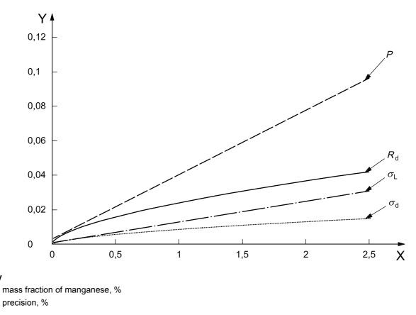
Figure C.1 — Least-squares fit of precision against *X* for manganese (alkali fusion)
