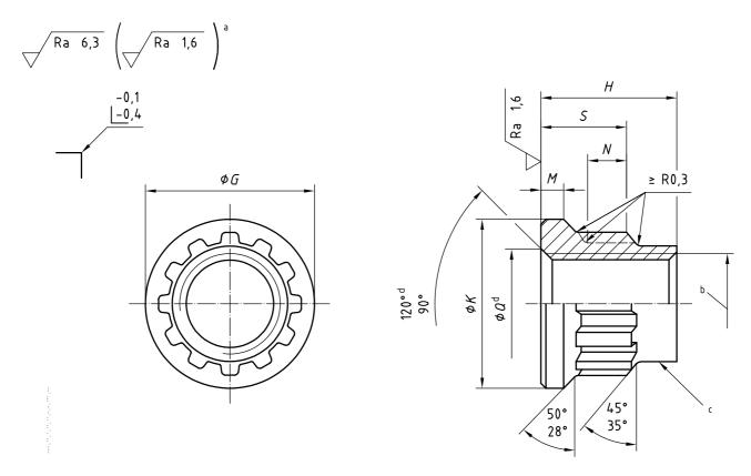
Tolerances of form and position shall conform to those specified in ISO 8788. Details of form not stated are at the manufacturer's discretion.
