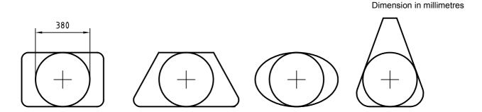
Figure 2 — Measurement of minimum clear opening
