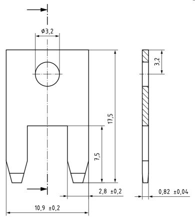
Where not specified in the figure, the common tolerances shall be in accordance with tolerance class m as specified in ISO 2768-1.
