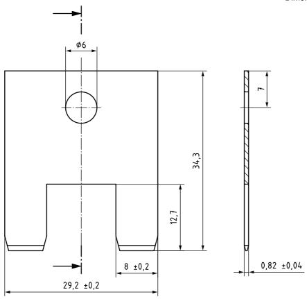
Where not specified in the figure, the common tolerances shall be in accordance with tolerance class m as specified in ISO 2768-1.
