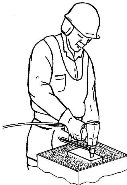
Figure 3 — Fastener driving tool — Working position of operator
