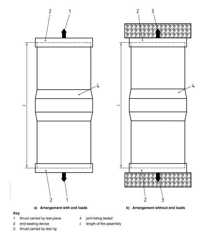
Figure 1 — Typical test arrangements for the tests detailed in 7.2, 7.3 and 7.5
