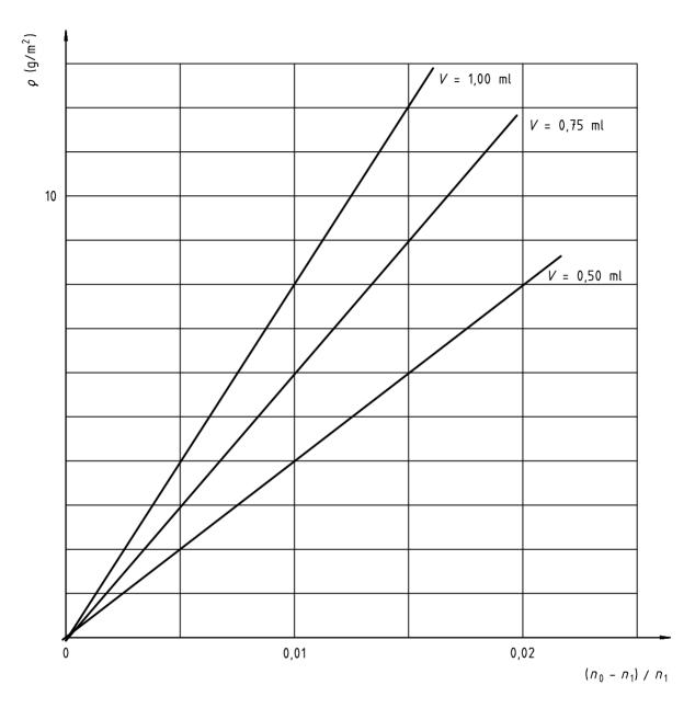
NOTE Each straight line corresponds to a different volume of solvent in the syringe. In each case the patch size is A-1250 as defined in ISO 8502-6.
