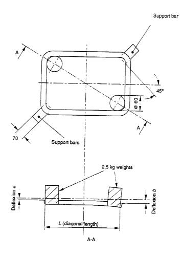
NOTE Corners of support bars are coincident with the edge of the flat base area
