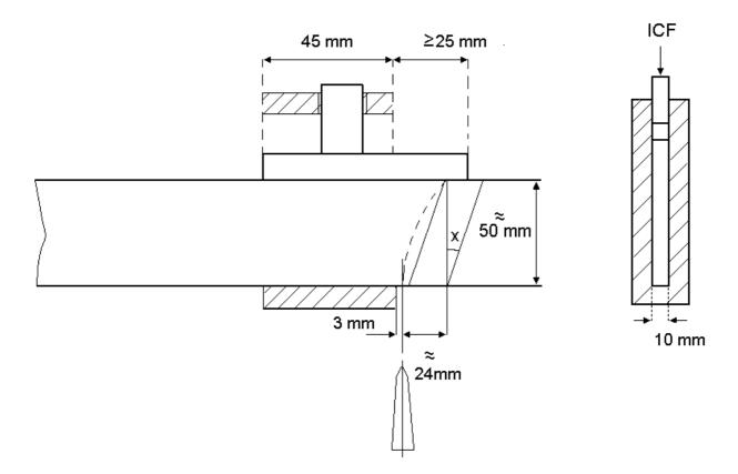
No test shall be performed within 25 mm of the start of the new pack.
