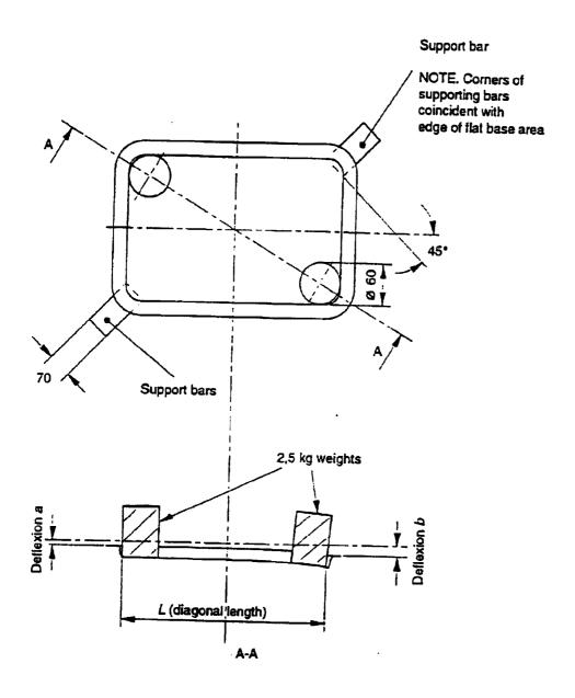
Figure E.1: Twist test for trays and dishes
