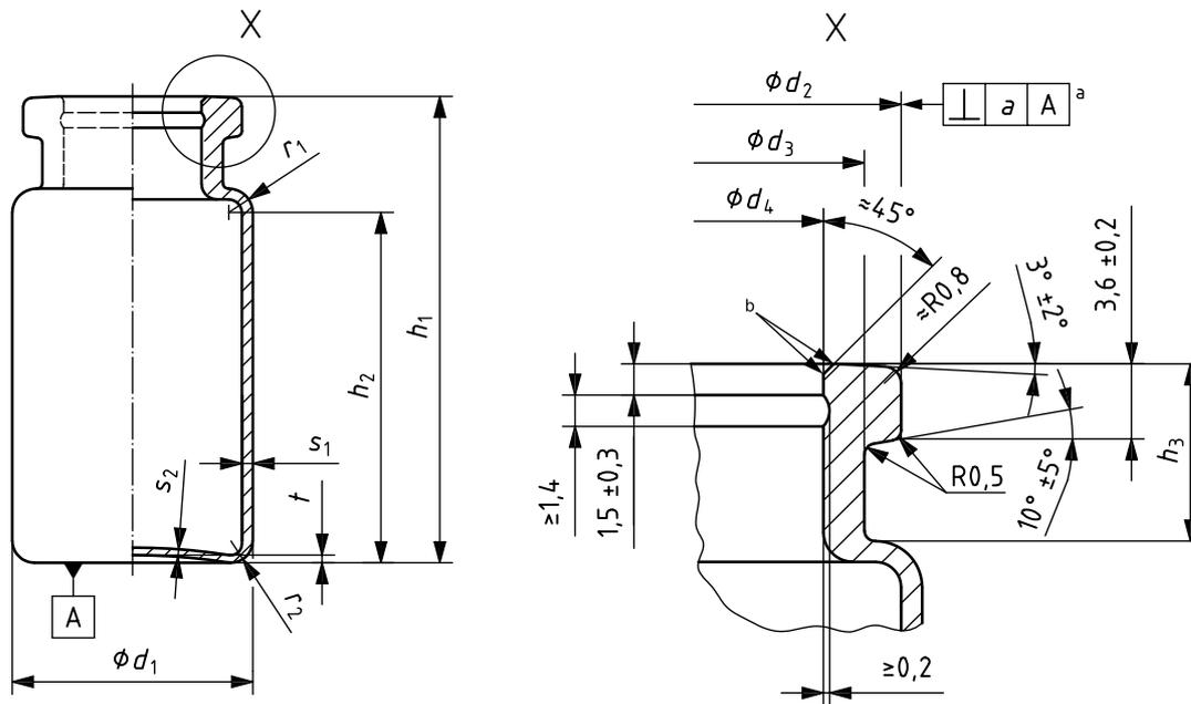
a The perpendicularity tolerance *a* (as defined in ISO 1101) is a limit for the deviation of the plumb-line through the centre of the bottom part and the axis of the vial at the upper edge of the flange; it is measured at the brim.
