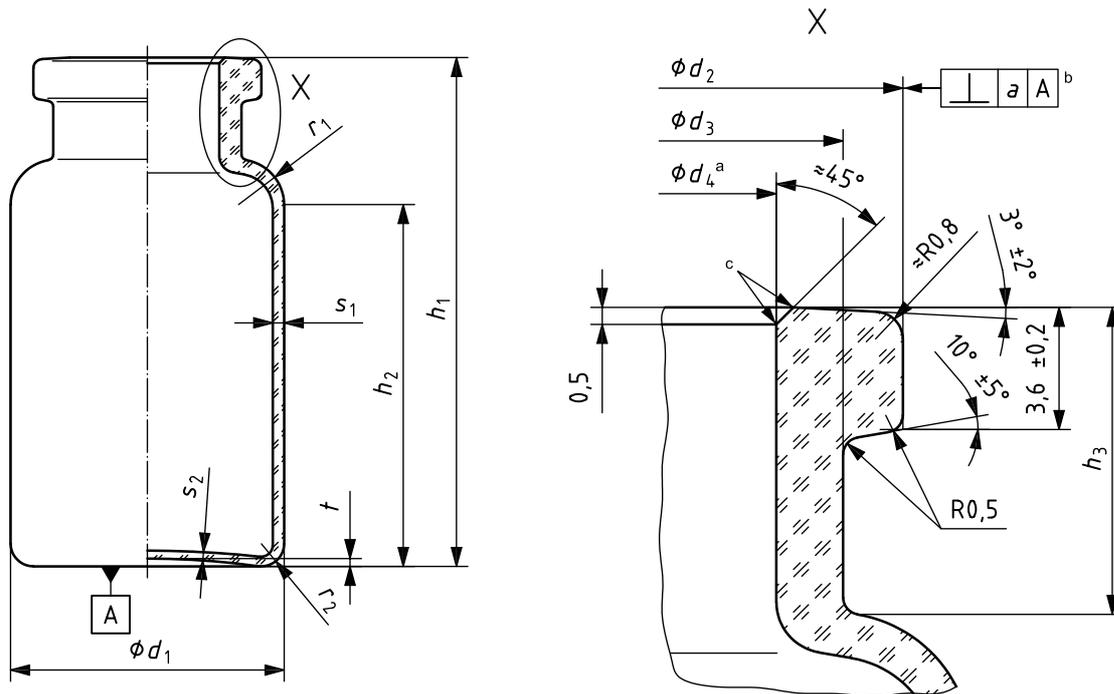
a The opening of the vial should have a constant diameter, over the entire distance,  $h_3$ , i.e. it should exhibit a cylindrical shape. A slightly conical shape can be accepted if the following requirements are fulfilled:
