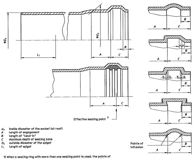
measurement for A and C shall be indicated by the manufacturer and these points shall give a full sealing action.
