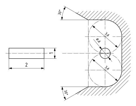
Required space envelope for clearance: 3A above and below the towing spool centre.
