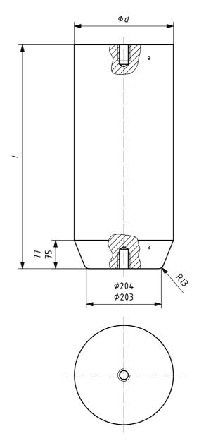
NOTE Dimensions d and l are optional, depending on the mass of the test object required to match the drop height that will provide the energy specified in 4.3.4. For example, for a drop test object mass of 227 kg:
