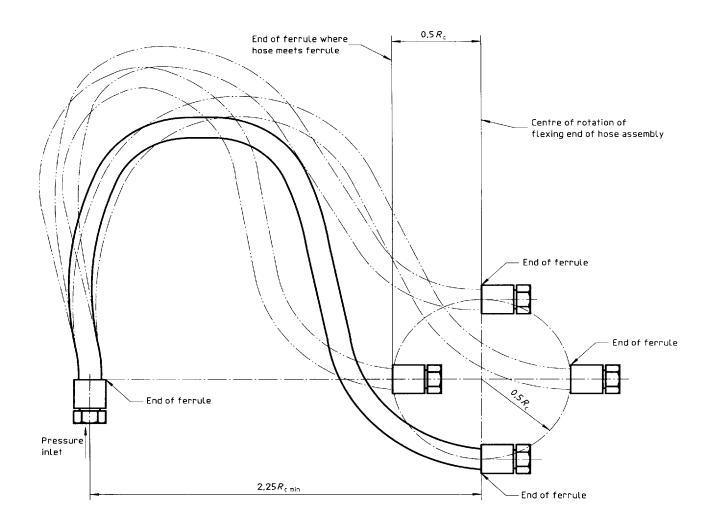
Figure 1 - Schematic arrangement of test piece
