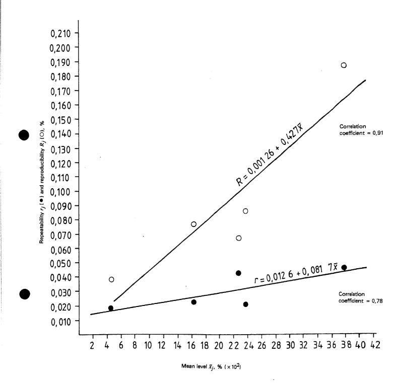
Figure — Graph of repeatability  $r_j$  and of reproducibility  $R_j$  as a function of mean level  $\bar{x}_i$
