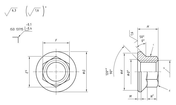
Tolerances of form and position shall conform to those specified in ISO 8788. Details of form not stated are at the manufacturer's discretion.
