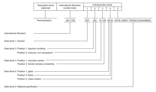
Specification: ISO 7792-PET,MC,07-140,GF45,ASTM D5927 TPES0210G45A88560
