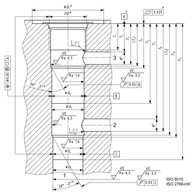
1, 2 and 3, ports PD (thread) pitch diameter
