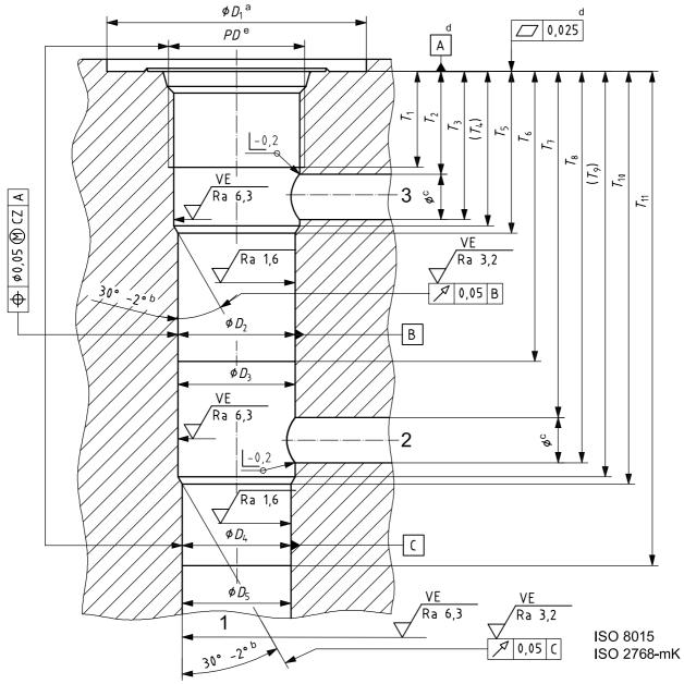
1, 2 and 3, ports PD (thread) pitch diameter NOTE The same designations are used in Table 14. VE visual examination
