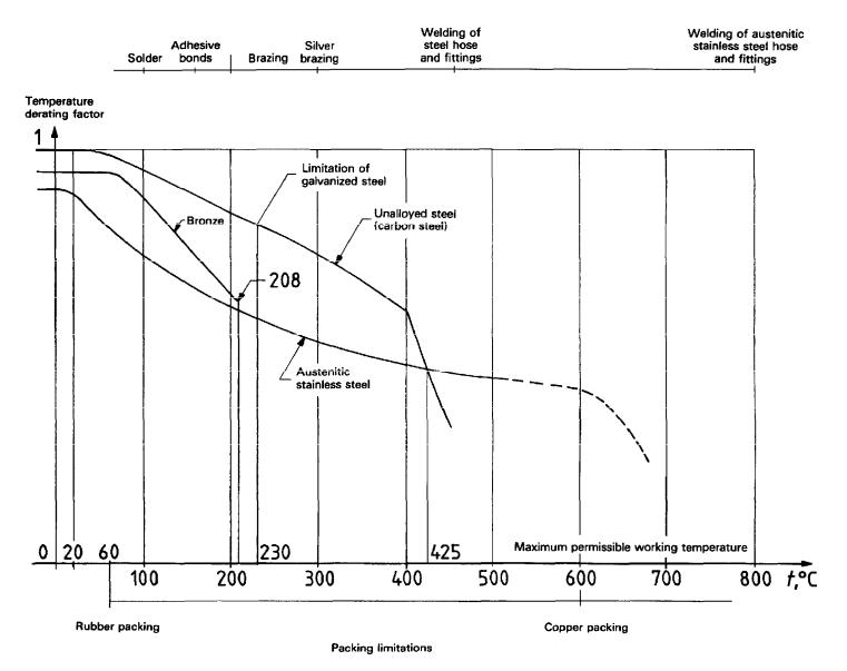
The temperature derating factor is the ratio of burst pressure at temperature t to burst pressure at room temperature. It is therefore equal to the ratio of maximum permissible working pressure at temperature t to the maximum permissible working pressure at room temperature.
