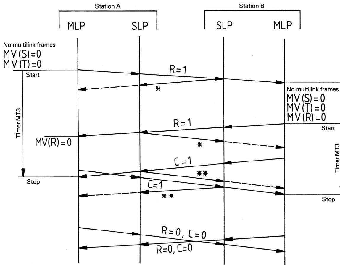
\* The SLP frame that acknowledges delivery of the multilink frame with  $R = 1$ .
