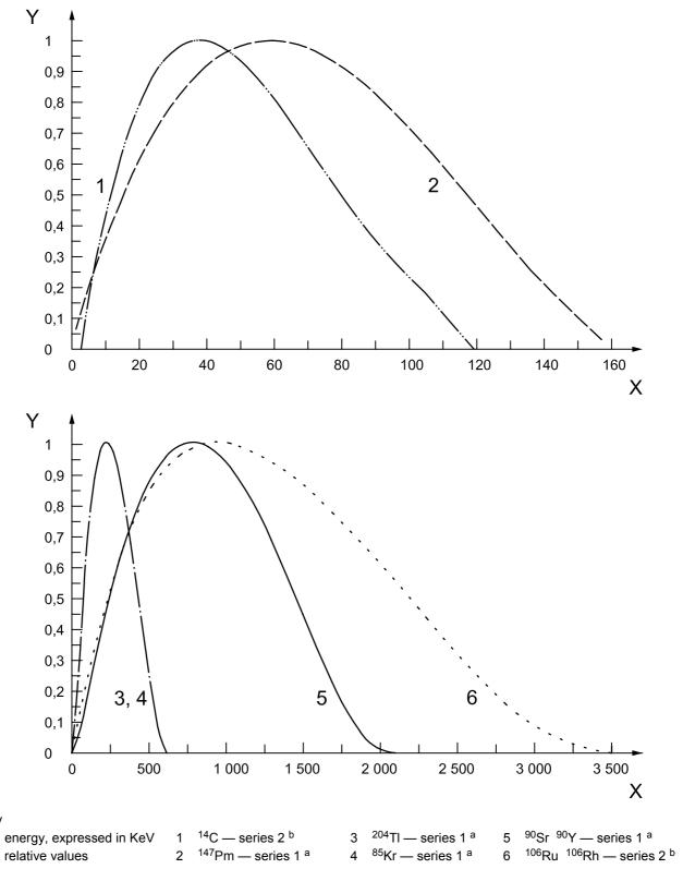
The spectra are measured with an effectively windowless, uncooled Si(Li) semiconductor detectors.
