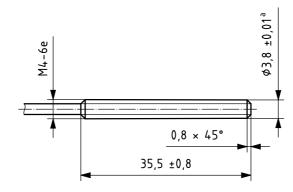
The gauge shall be of hardened steel.
