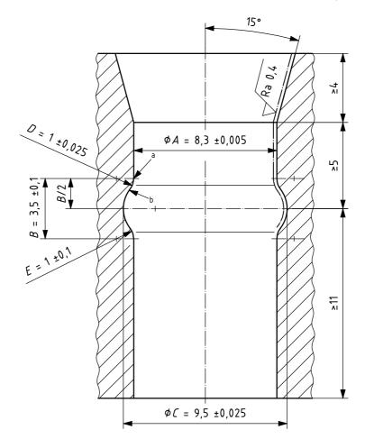
The gauge shall be of hardened steel.
