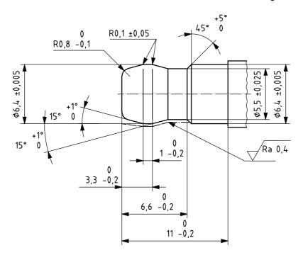
The gauge shall be of hardened steel.
