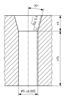
The gauge shall be of hardened steel.
