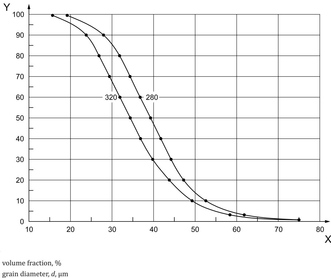
**Figure 3 — Cumulative volume grain size distribution curve of checking minerals 280 and 320**
