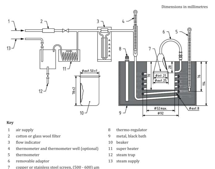
Figure 1 — Apparatus for determining gum content by jet evaporation
