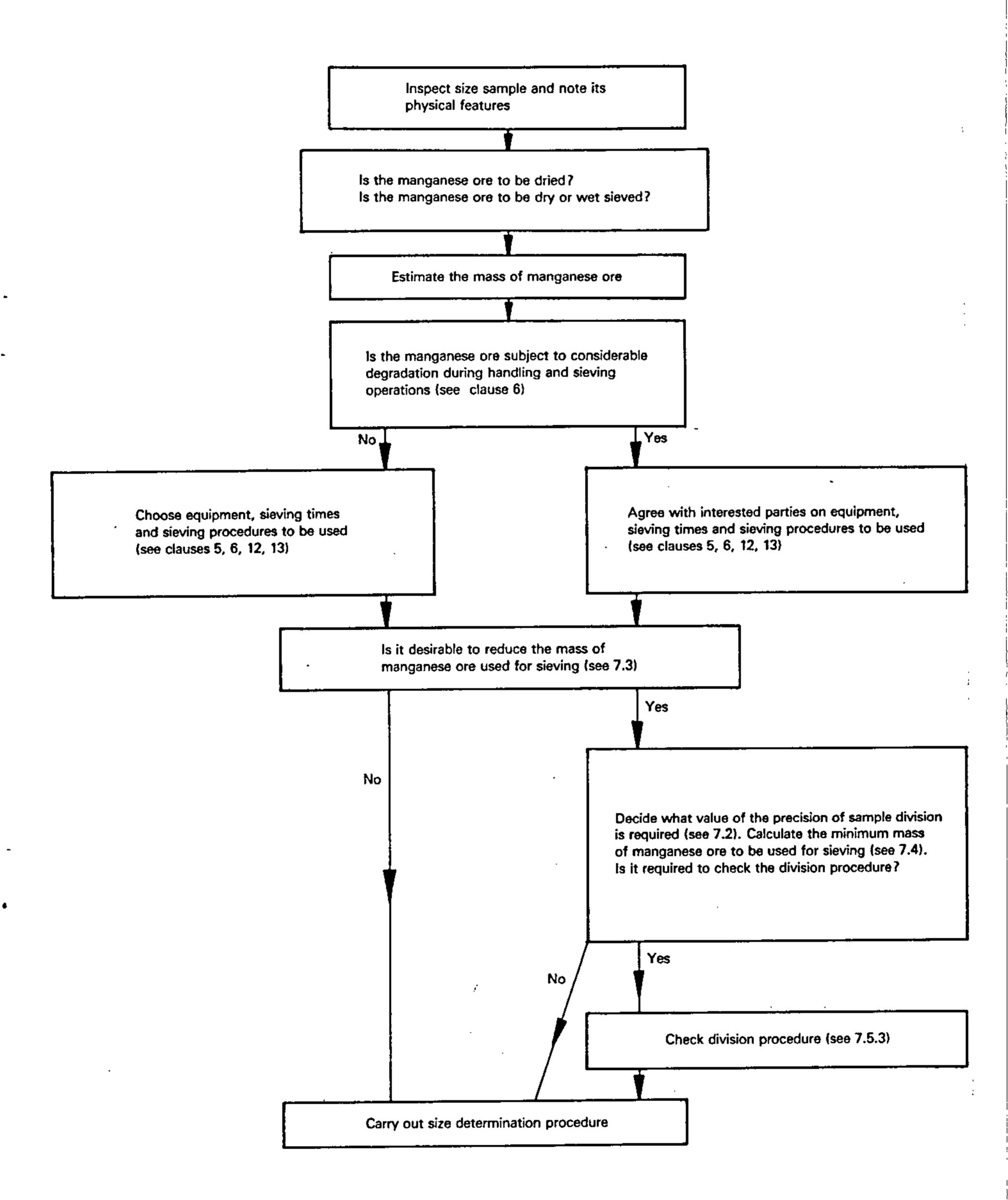
Figure 2 - Typical decision tree for selecting size determination procedure
