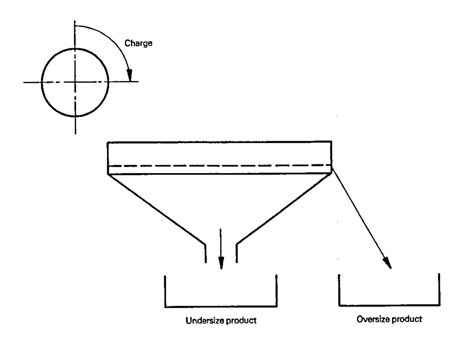
Figure 3 — The scheme of continuous sieving equipment
