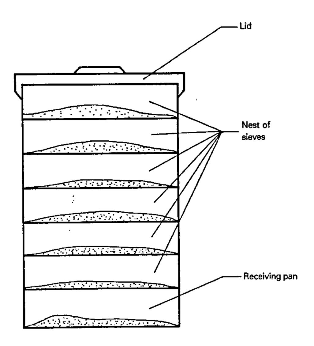
Figure 4 — The scheme of batch sieving apparatus
