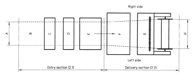
A = width of entry warpH = width of delivered warp
