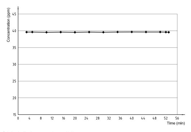
Calculated calibration concentration: 39,63 ppm Average measured value: 39,60 ppm
