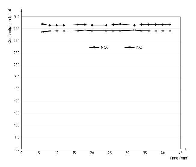
Calculated calibration concentration for NO<sub>x</sub>: 299 ppb
