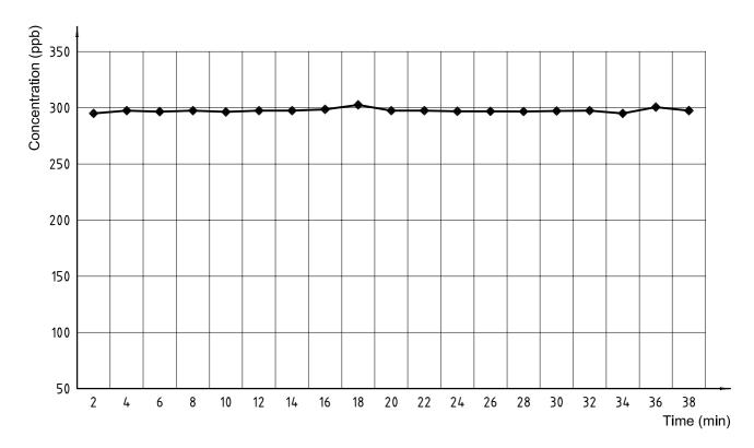
Calculated calibration concentration: 299 ppb 297,5 ppb Average measured value:
