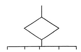
10.3.1.2 Each exit from a symbol should be accompanied by the appropriate condition values to show the logic path which it represents, so that the conditions and the associated references are identified.
