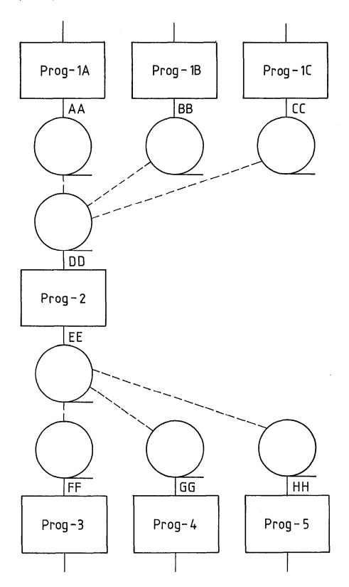
b) an output which is used as an input in a succeeding process will be connected to the input by a dashed line.
