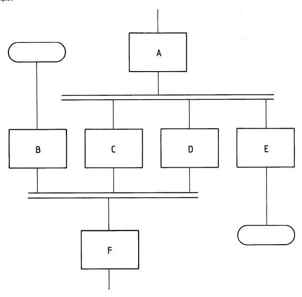
NOTE — Processes C, D and E cannot commence until process A has been completed; similarly process F should await completion of B, C and D; but process C may start and/or end before process D has started and/or ended respectively.
