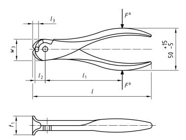
F =Load applied in load test or  $F_1$  force applied in cutting test.
