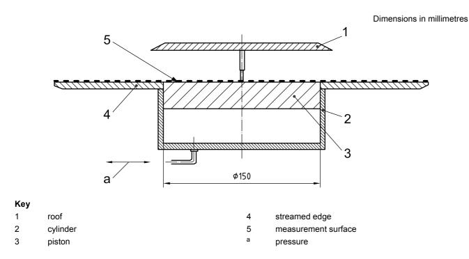
Figure B.5 — Plate sediment trap in its open state (schematic)
