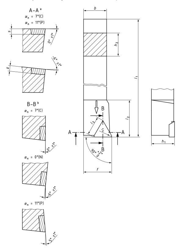
NOTE The figure shows a right-hand tool holder (R); left-hand tool holder (L) laterally reversed.
