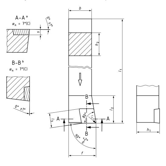
NOTE The figure shows a right-hand tool holder (R); left-hand tool holder (L) laterally reversed.
