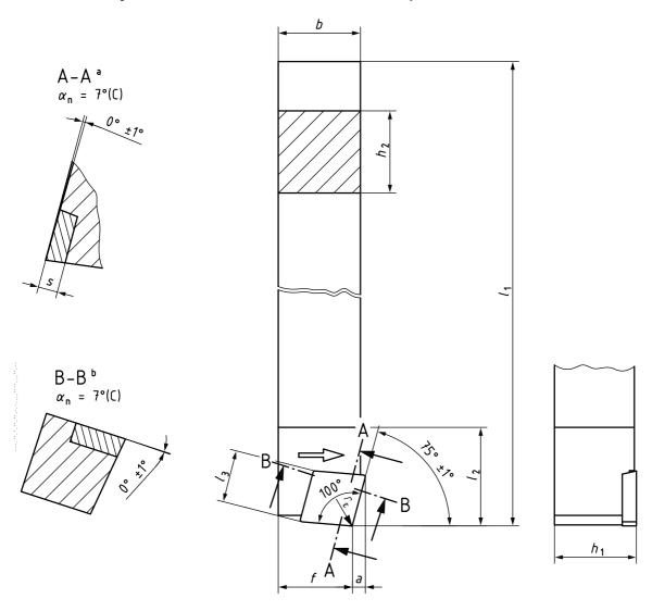
NOTE This figure shows a right-hand tool holder (R); left-hand tool holder (L) laterally reversed.
