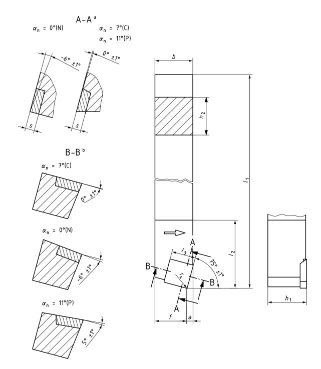
NOTE This figure shows a right-hand tool holder (R); left-hand tool holder (L) laterally reversed.
