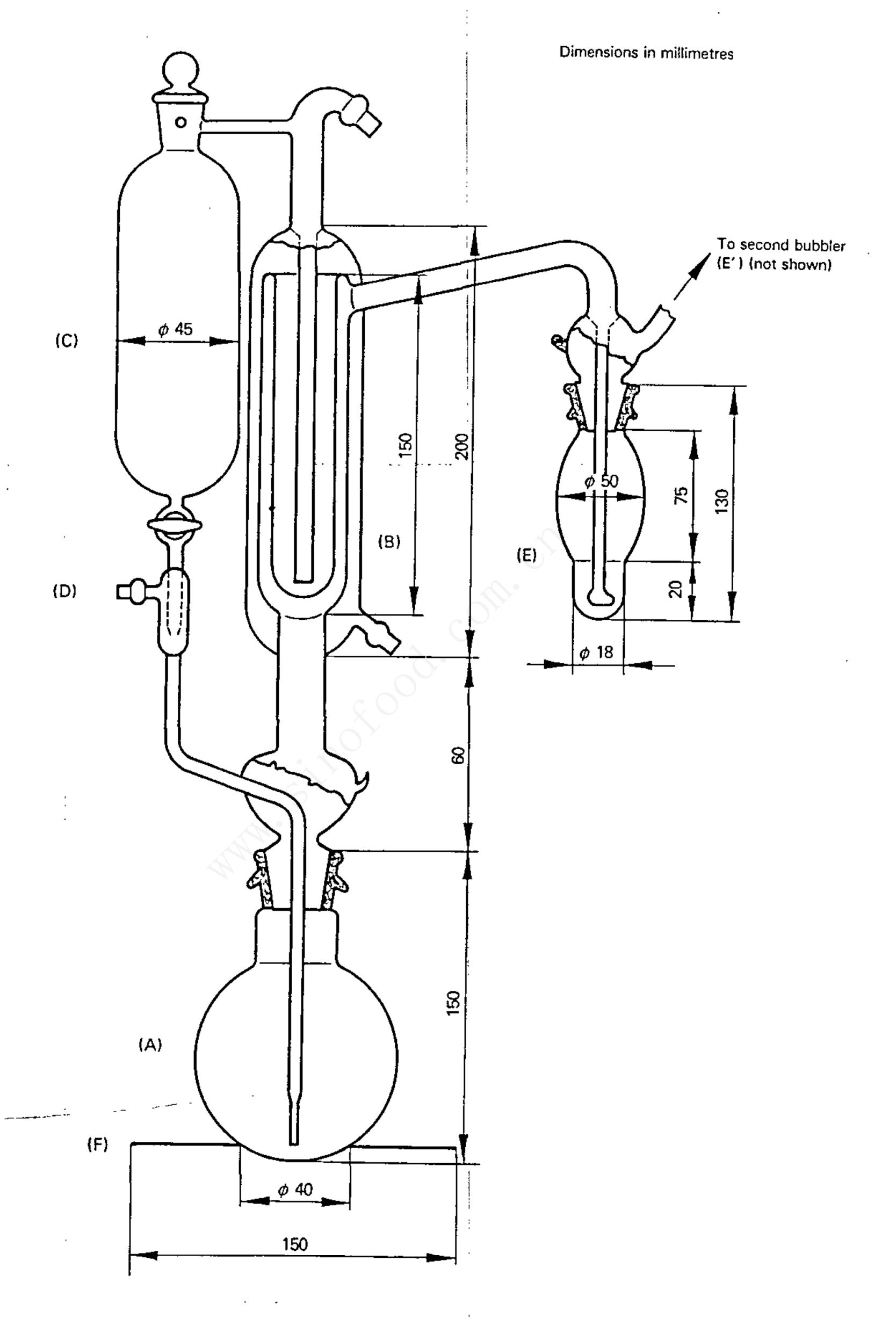
NOTE — The internal diameters of the four concentric tubes which serve as the condenser are 45, 34, 27 and 10 mm, respectively. It is advantageous to replace the two ground conical surfaces by spherical ones.
