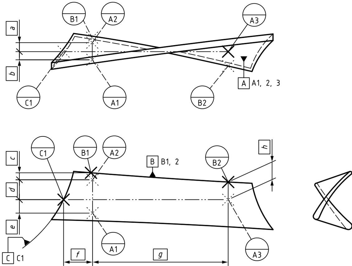
Figure 28 — Example of indications of datum targets on complex surfaces
