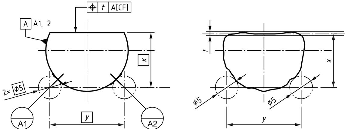
**Figure A.6 — Examples of single datums established on a nominally cylindrical surface, with [CF] (contacting feature) modifier, used in a geometrical specification**
