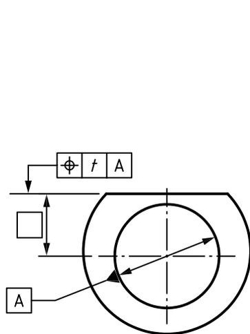
NOTE The associated feature used to establish the datum from the complete integral feature is a cylinder and the datum is its axis.
