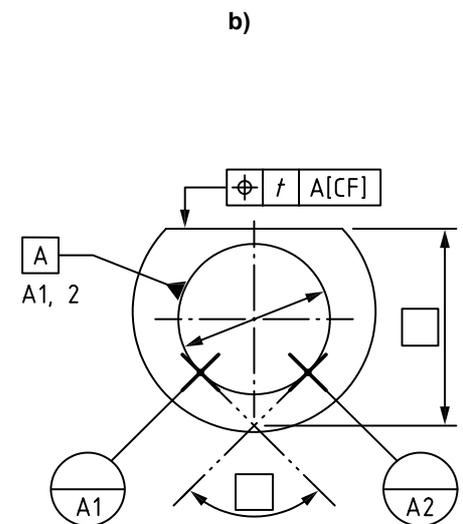
NOTE The datum targets A1 and A2 are defined by the interface between the cylinder A and a contacting feature. The distance between datum targets A1 and A2 is variable. It depends of the actual diameter of the cylinder and the contacting feature defined in this case by a "V" block of angle  $\alpha$ . The associated feature used to establish the datum is the "V" block, not a cylinder.
