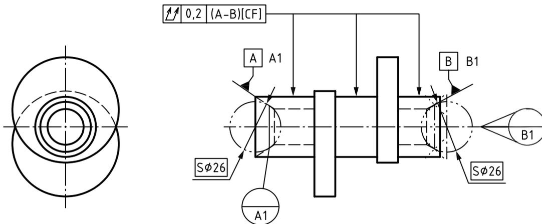
Figure 30 — Example of datum system in which the datum target is indicated
