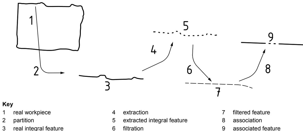
**Figure A.1 — Example of procedure to establish an associated feature**
