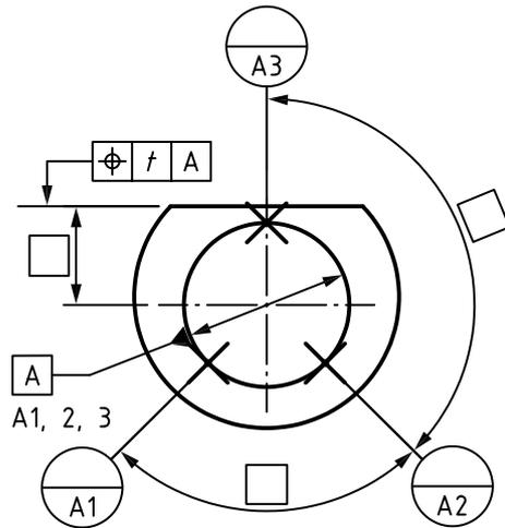
NOTE The angular locations between the datum target lines A1, A2 and A3 are indicated by TEDs and are considered as fixed. The associated feature used to establish the datum from 3 datum target lines is a cylinder and the datum is its axis.
