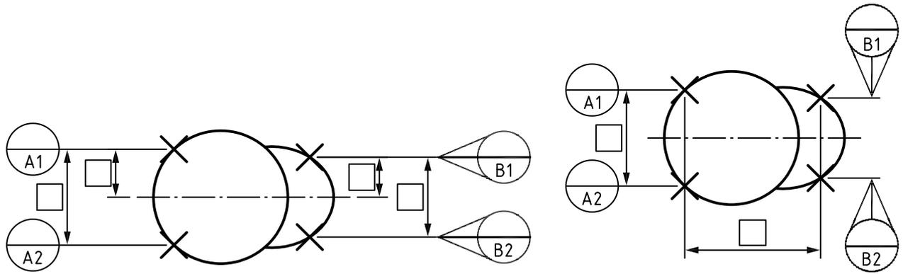
NOTE The motion of the moveable datum target, which is given by the direction of the moveable modifier, is perpendicular to a line going through the datum targets A1 and A2.
