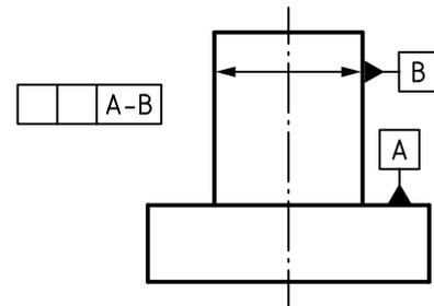
**Figure C.27 — Plane and perpendicular cylinder — Input for reading (drawing indication) and for writing (design intent)**
