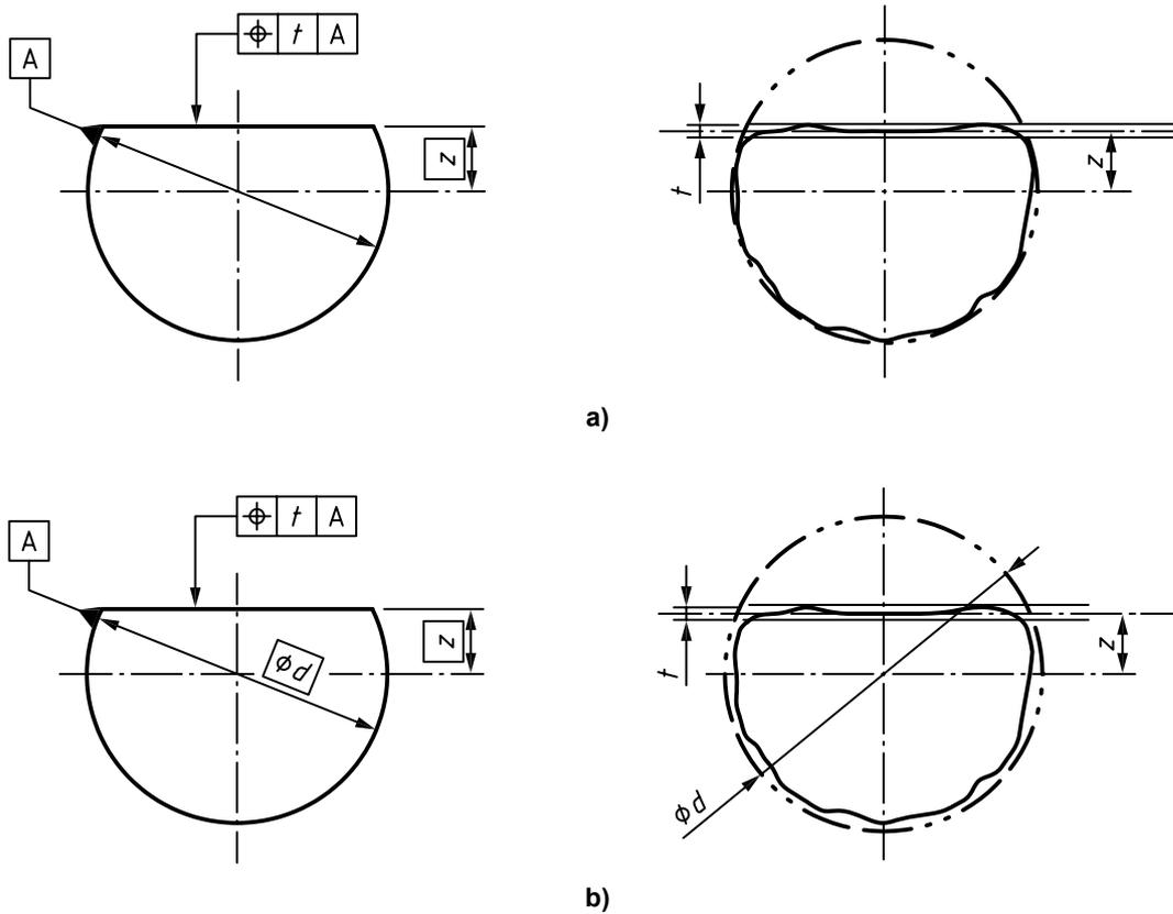
NOTE When associating a cylinder of fixed size, the maximum distance between the associated cylinder and the real (extracted) cylinder is minimized, without orientation, location and material constraints.
