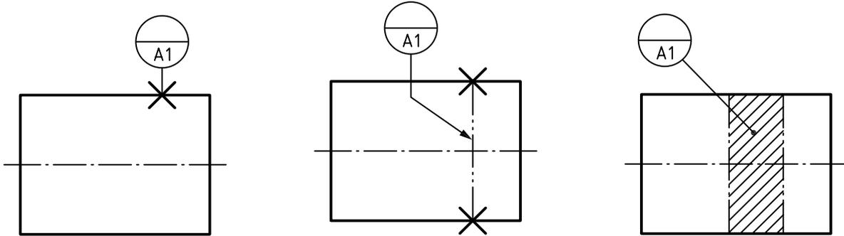
Figure 12 — Indicator for single datum target point
