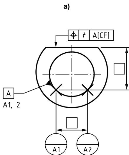
NOTE The distance between datum targets A1 and A2 is indicated by a TED and is fixed. The associated feature used to establish the datum is not a cylinder and the datum is not its axis. The datum consists of two planes: one plane through two datum target lines and a second perpendicular median plane.
