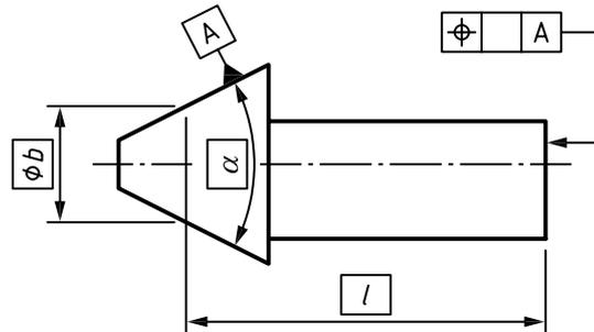
NOTE This particular point is defined by the intersection between a plane and the axis of the cone. This plane is perpendicular to the axis of the cone and its location defined by the TED  $\phi b$  that defines the diameter of a circle. This circle is the intersection between the associated cone and the plane.
