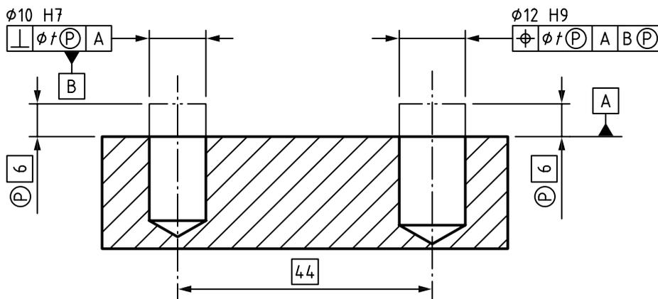
Figure 39 — Example of application of modifier  $\text{\textcircled{P}}$  on the secondary datum
