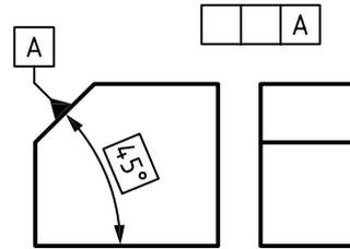
**Figure C.17 — Intersecting planes — Input for reading (drawing indication) and for writing (design intent)**
