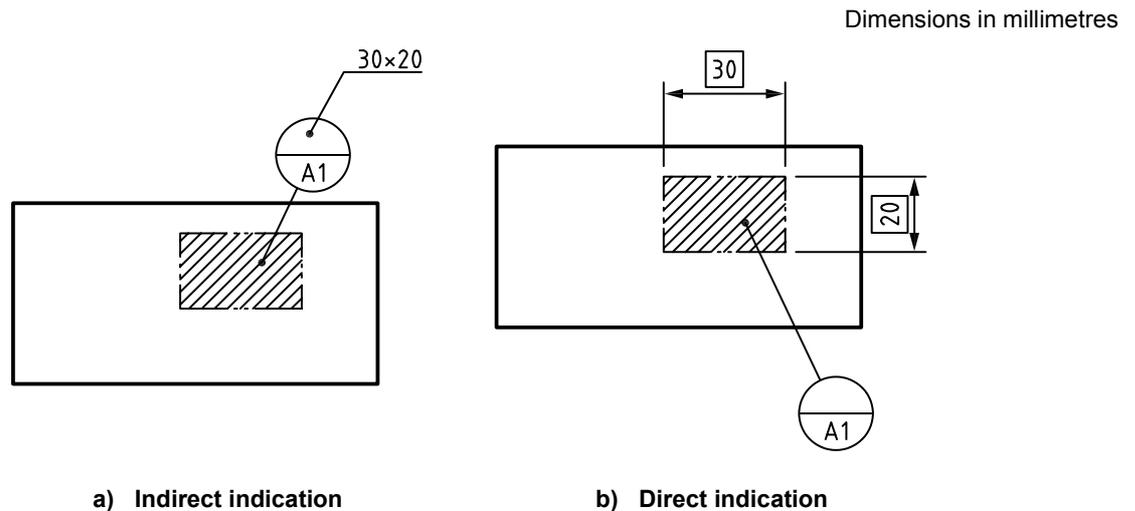
**Figure 25 — Indication of dimensions of a rectangular area**
