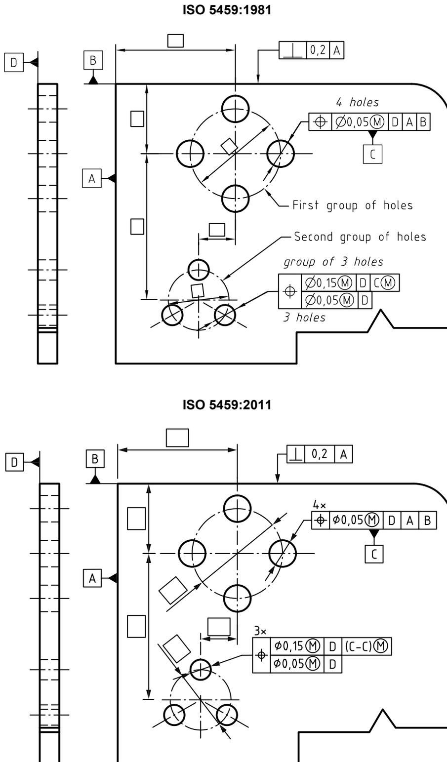
Figure D.3 — Indication of a common datum
