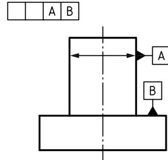
**Figure C.38 — Cylinder and perpendicular plane — Input for reading (drawing indication) and for writing (design intent)**
