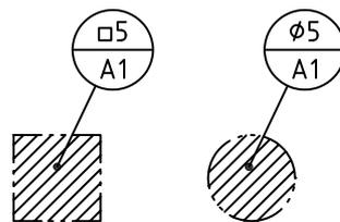
Figure 24 — Indication of dimension of a circular/square area
