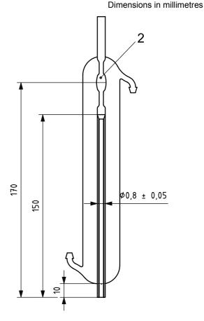
b) Viscometer for determining viscosities of test solutions
