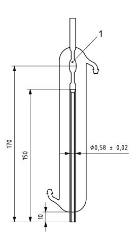
a) Viscometer for calibration
