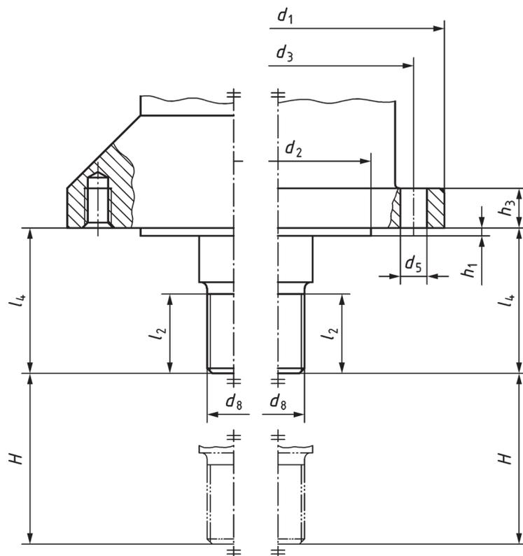
Figure 10 — Dimensions of linear output drive
