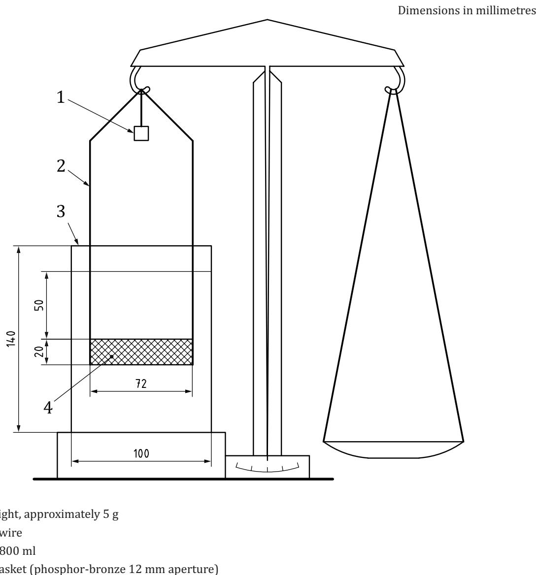
**Figure 1 — Modified beam balance**
