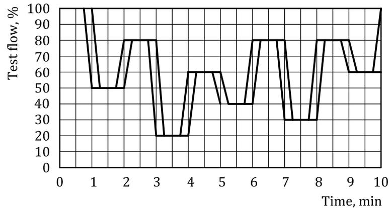
Figure 1 — Typical variable flow cycle (average flow 60 %)
