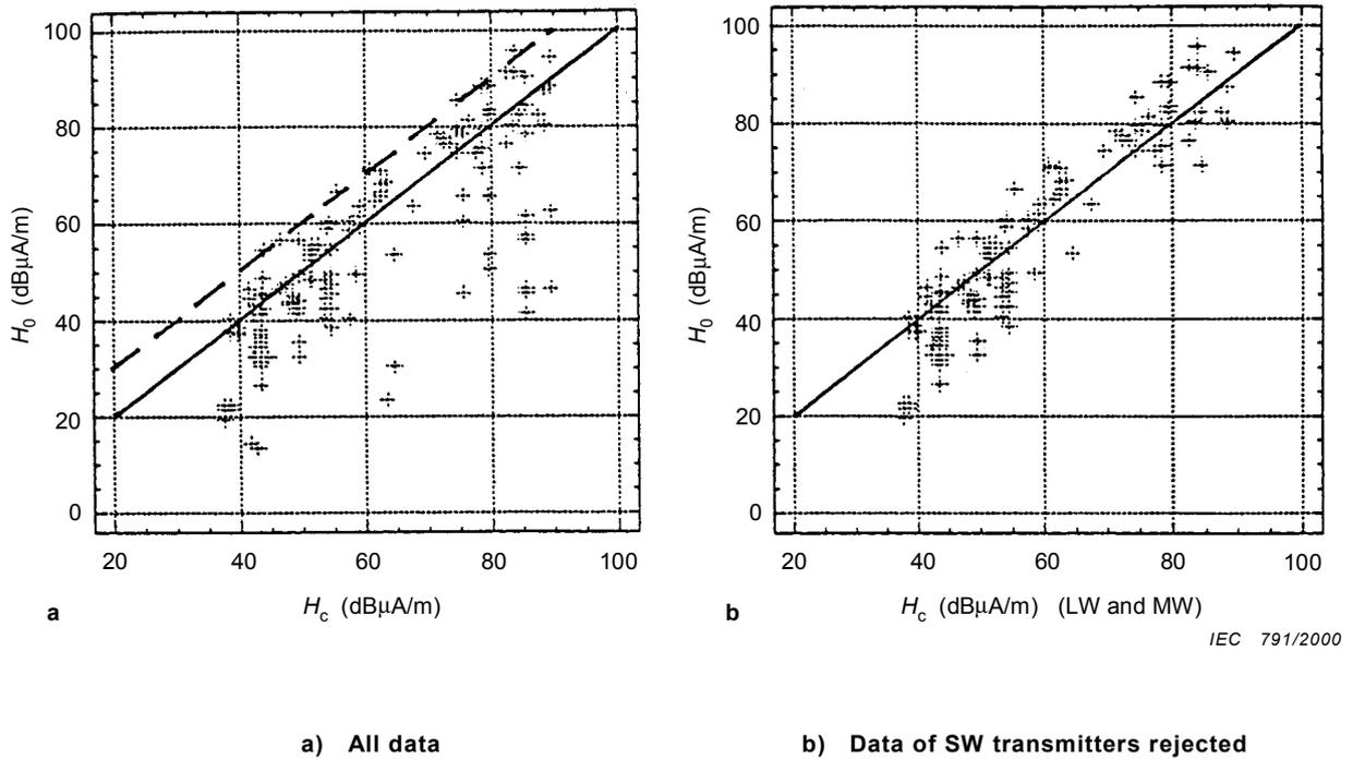
**Figure 7 – Scatter plot of the measured outdoor magnetic field strength  $H_o$  (dB $\mu$ A/m) versus the calculated outdoor magnetic field strength  $H_c$  dB( $\mu$ A/m)**
