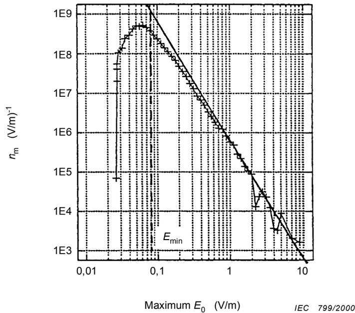
NOTE The solid line represents  $n(E_o) = -C_{E_o}/E_o^3$  with  $n(E_o = 1 \text{ V/m}) = n_m(E_o = 1 \text{ V/m}) \times E_{\min}$  chosen such that the integral over the field strength of  $n_m(E_o)$  and  $n(E_o)$  both yield the total number of outlets in that region.
