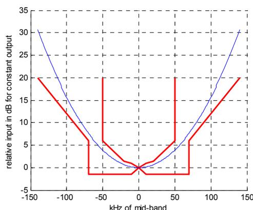
**Figure 191 – Example of a 120 kHz Gaussian filter**
