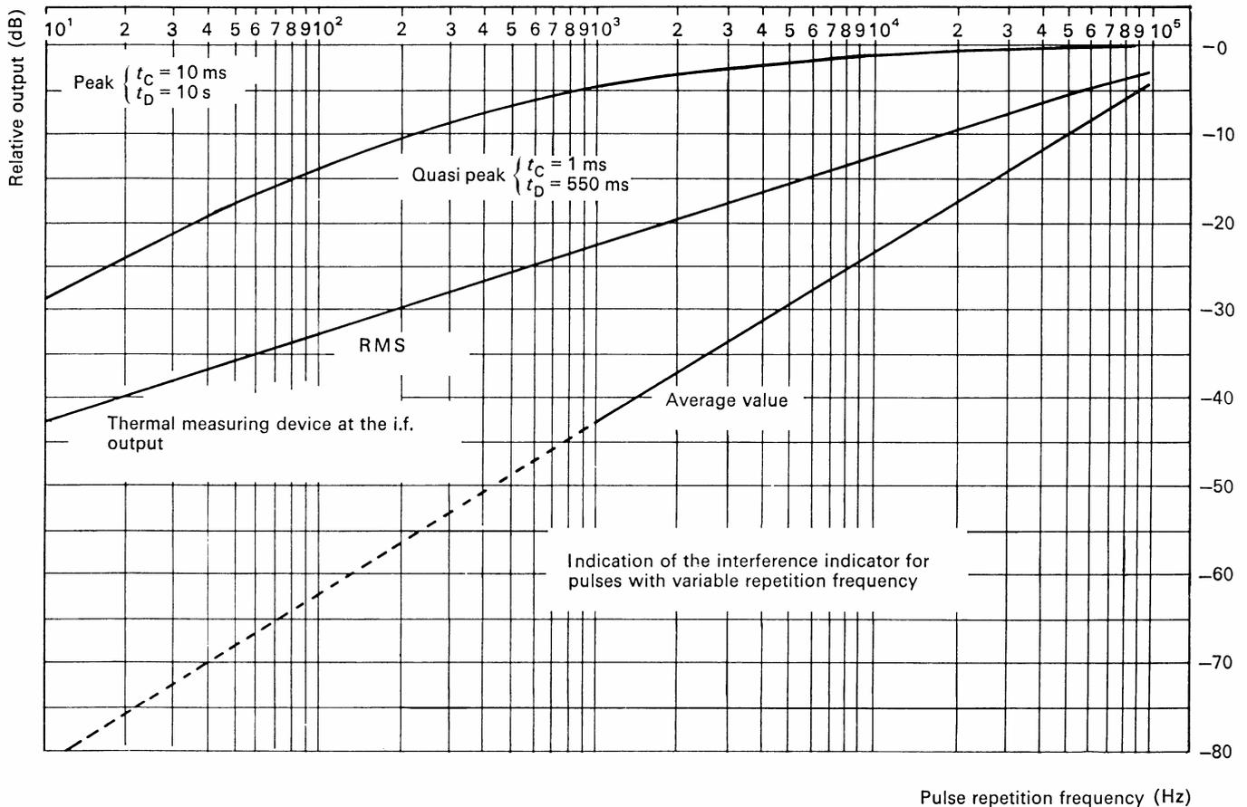
**Figure 1 – Relative response of various detectors to impulse interference**
