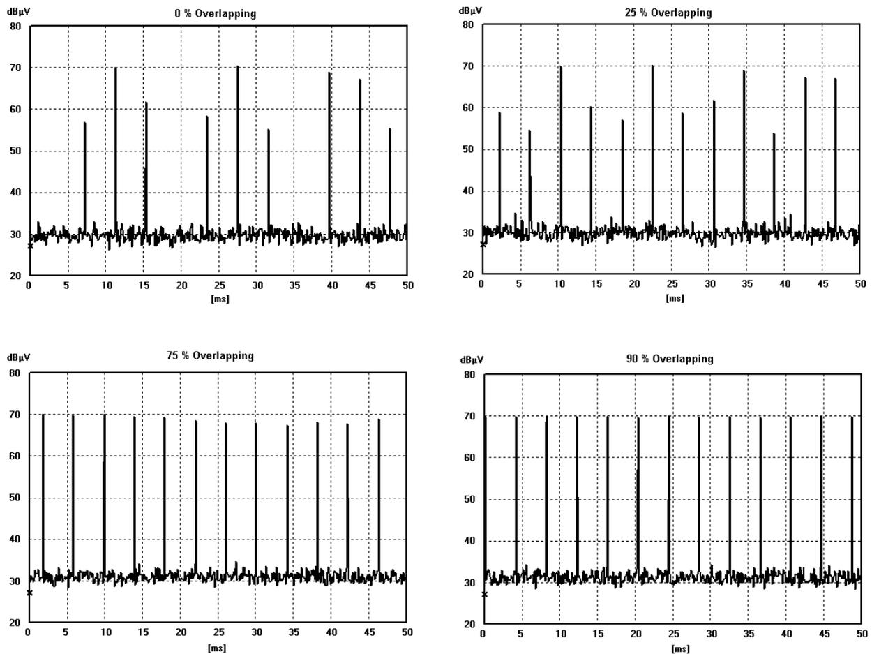
Figure 185 – IF signal for different overlapping factors for the same sequence of pulses
