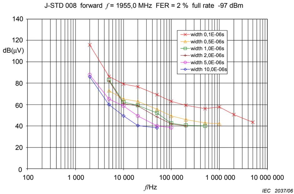
**Figure 165 – Weighting characteristics for J-STD 008 (signal level -97 dBm)**
