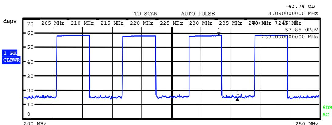
**Figure 193 – Dynamic range for broadband emission as measured with the peak detector**
