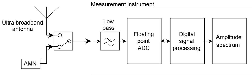
**Figure 186 – FFT-based baseband system**
