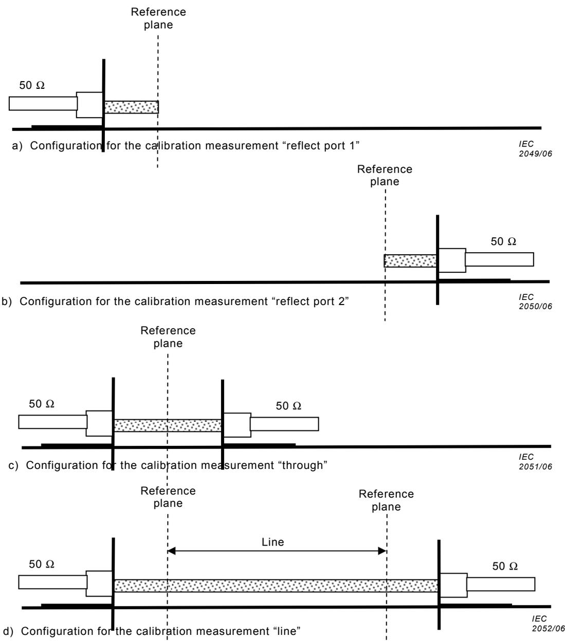
NOTE The length  $L$  of the reference line for the calibration needs not to be the same as the length used for the measurement of the CMAD. The length of the reference line for the calibration procedure has to be selected according to the frequency range needed.
