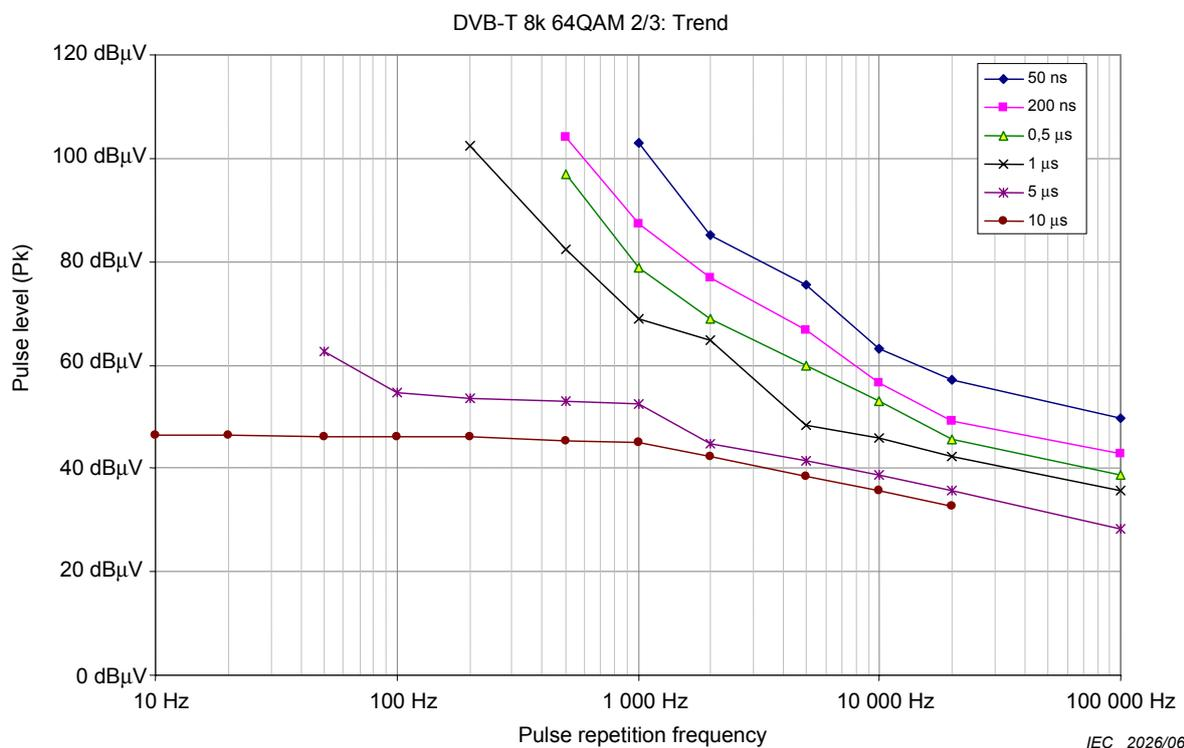
**Figure 154 – Average weighting characteristics of 6 receiver types for DVB-T with 64QAM**
