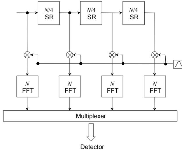
**Figure 189 – Short time fast Fourier transform – An example of implementation**
