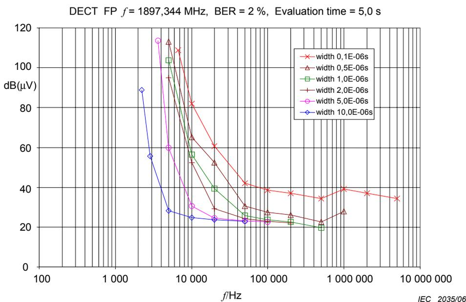
**Figure 163 – Weighting characteristics for DECT (signal level –83 dBm)**
