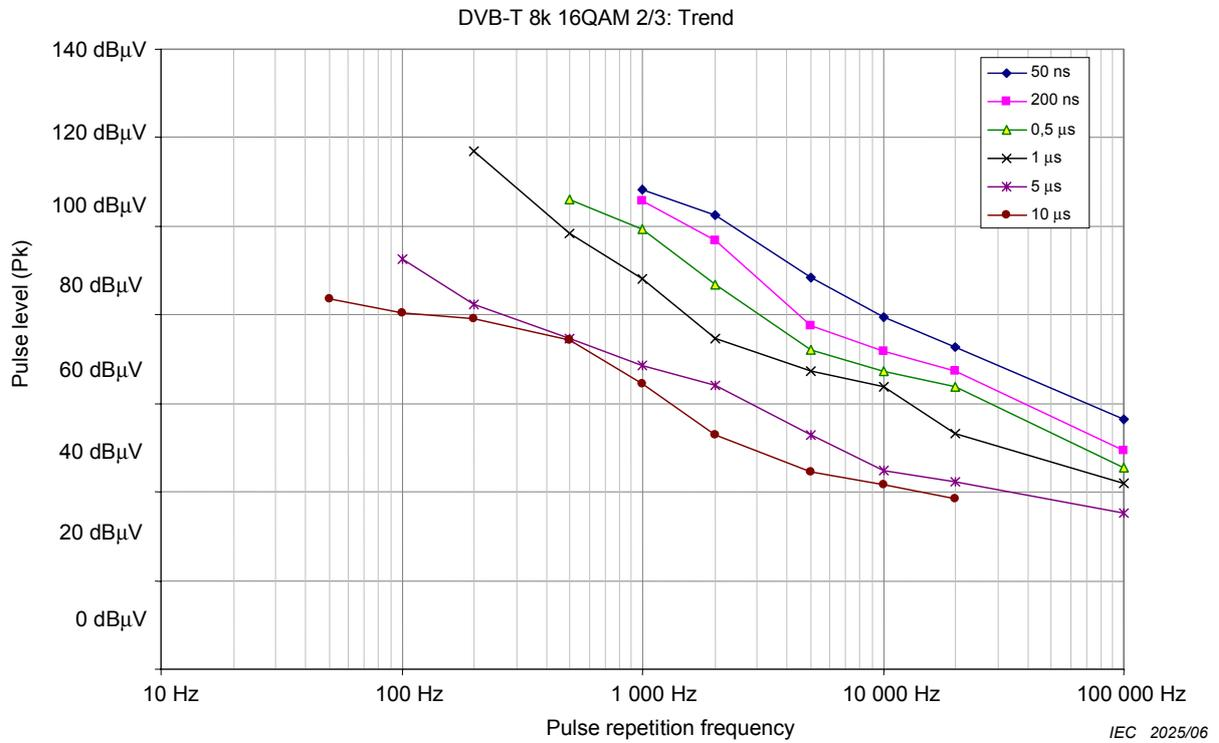
Figure 153 – Average weighting characteristics of 6 receiver types for DVB-T with 16QAM
