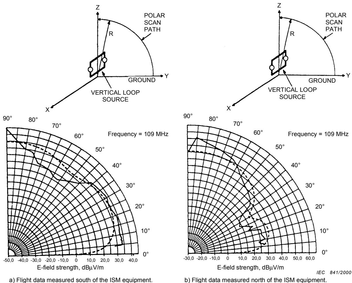
Solid curves: Machine D (fundamental RF power 2 kW), 20° azimuth, flight altitude 152 m, RF shields in place, derived from in-flight field strength data in Figure A-19 at page 72 in [33].
