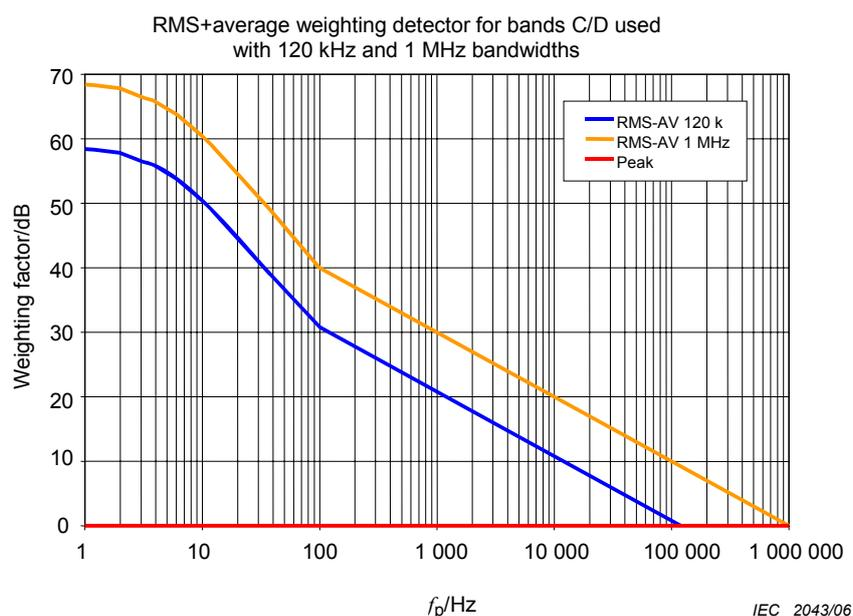
**Figure 171 – Shift of the rms-average weighting function for CISPR band C/D by using a bandwidth of 1 MHz instead of 120 kHz, if the shortest possible pulse widths are applied**
