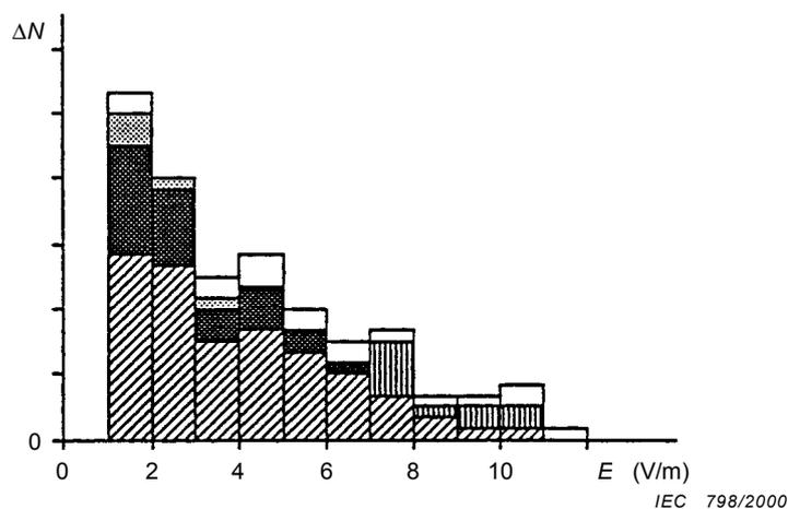
NOTE The various shadings indicate schematically the contributions from various transmitters and non-homogeneous outlet densities; in this example the field-strength increment is  $\Delta E_o = 1$  V/m.
