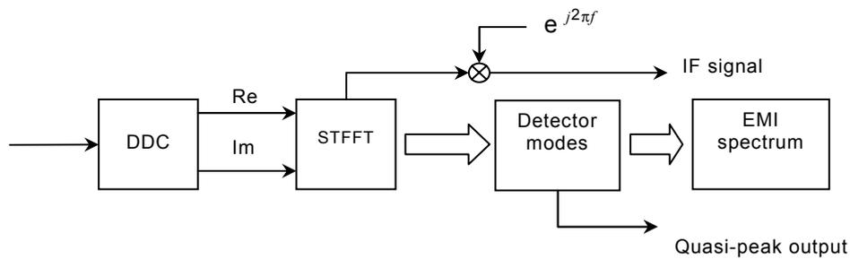
**Figure 187 – Real-time FFT-based measuring instrument**
