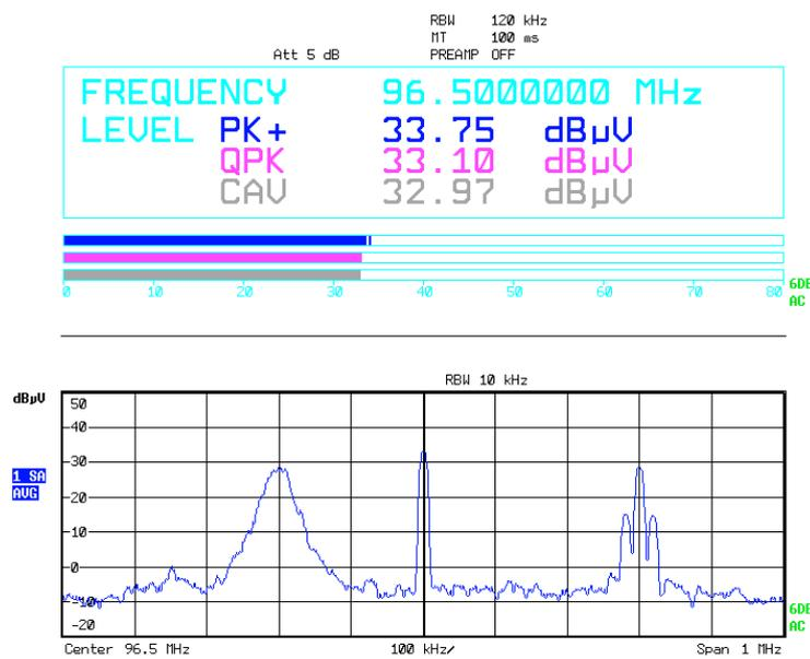
Figure 199 – Example FFT IF analysis display
