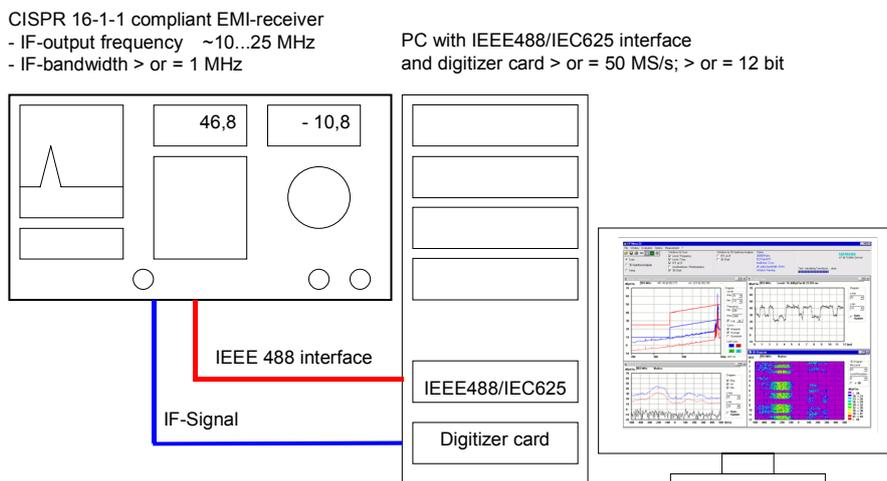
**Figure 194 – Set-up of FFT-based system type 2**
