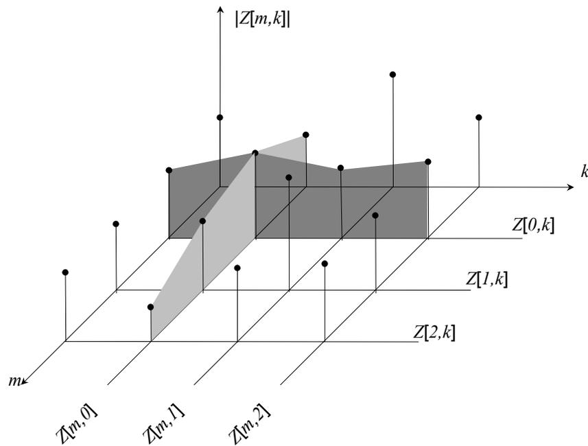
**Figure 182 – An example spectrogram  $Z[m,k]$**
