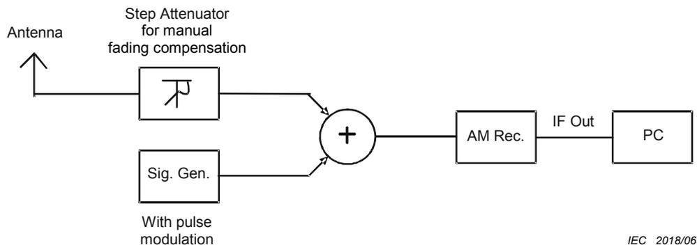
NOTE The received signal is downconverted to an IF of 12 kHz for decoding by special hardware and software in a personal computer (PC).
