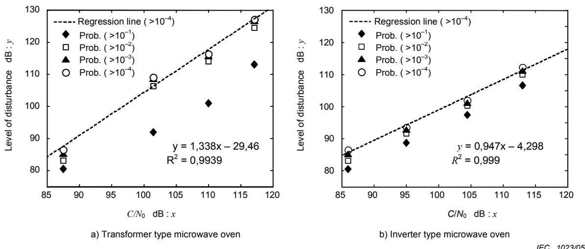
**Figure 128 – Correlation of the disturbance voltages with the system performance ( $C/N_0$ )**
