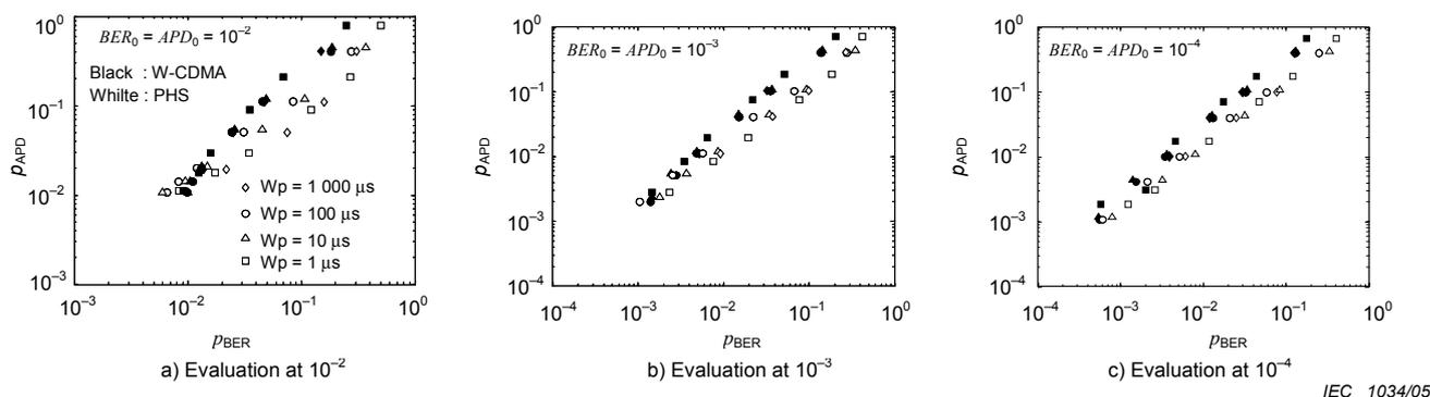
**Figure 139 – Correlation between measured  $p_{BER}$  and  $p_{APD}$**
