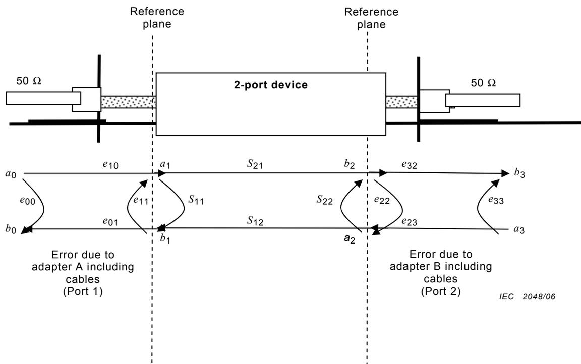
**Figure 176 – Basic model for the TRL calibration**
