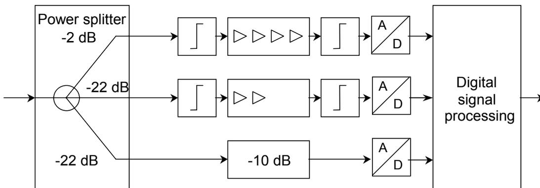
**Figure 190 – Floating-point analogue-to-digital conversion**
