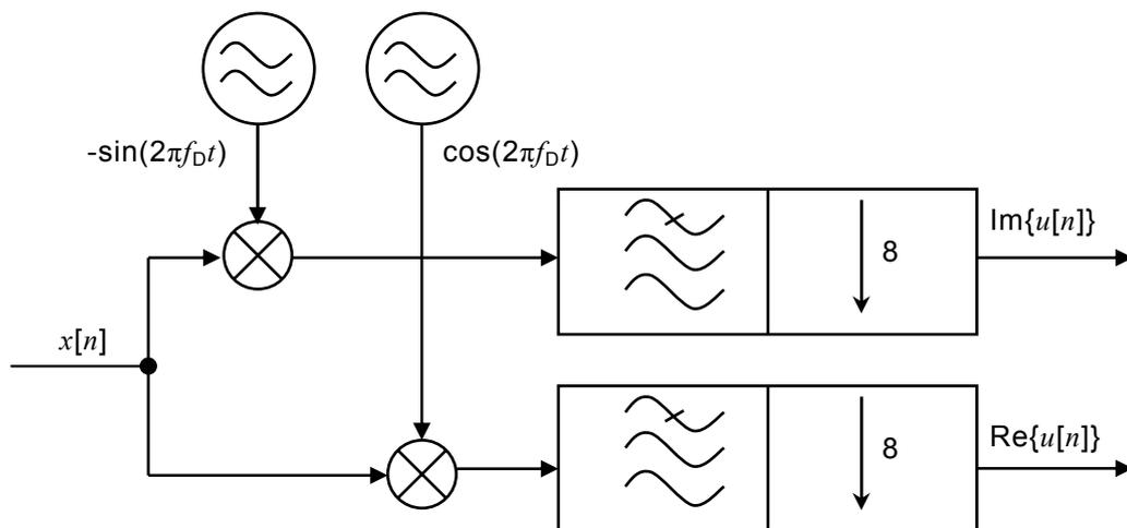
**Figure 188 – Digital down-converter**
