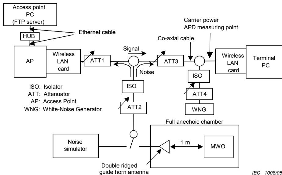
**Figure 113 – Set-up for measuring communication quality degradation of a wireless LAN**
