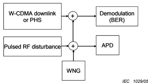
**Figure 134 – Simulation set-up for estimating communication quality degradation of a PHS or W-CDMA**
