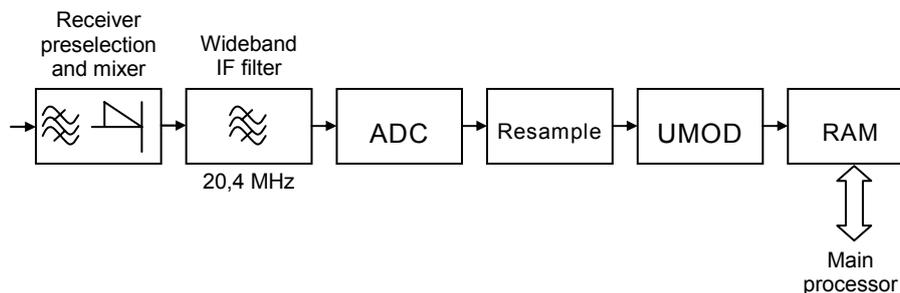
**Figure 192 – Essential parts of an FFT-based heterodyne receiver**
