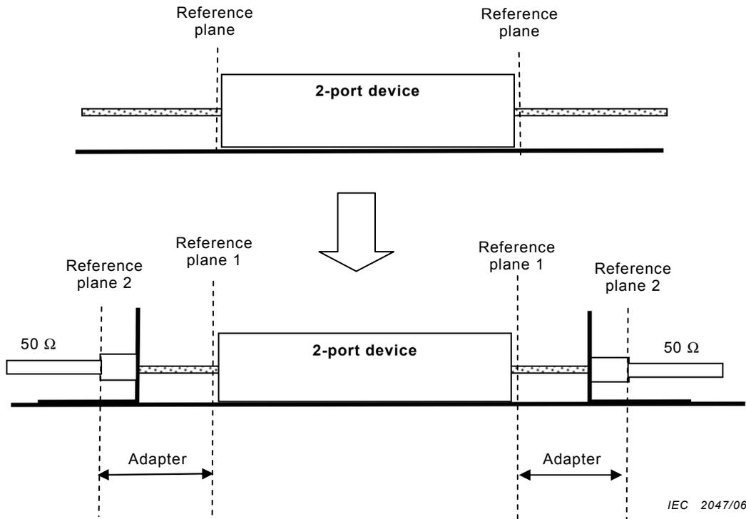
**Figure 175 – Conversion from 50 Ω coaxial system to the geometry of the two-port device-under-test**
