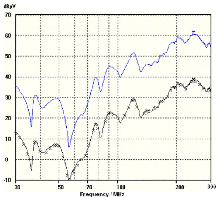
**Figure 196 – Example of pulse generator measurement with antenna**
