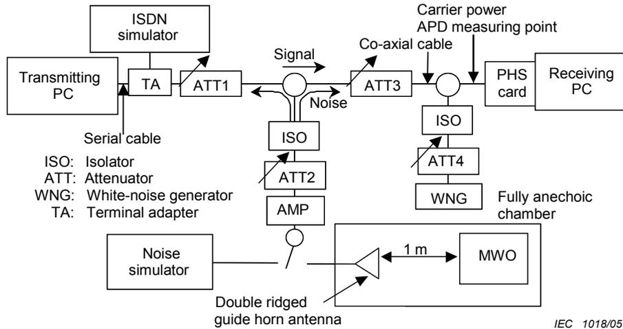
Figure 123 – Set-up for measuring the PHS throughput
