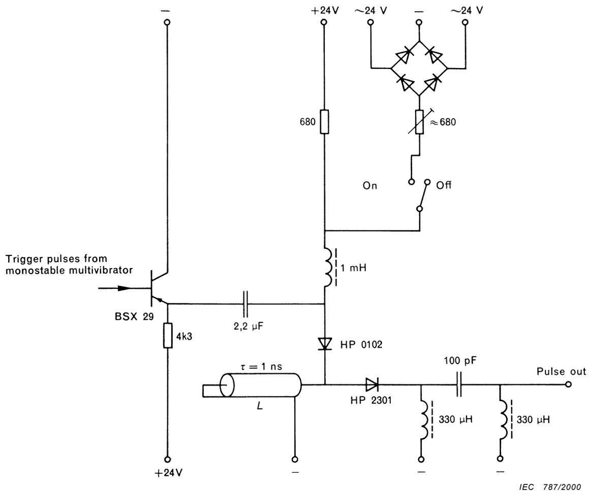
Figure 6 – Details of a typical output stage
