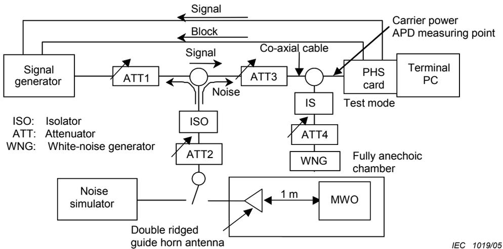
Figure 124 – Set-up for measuring the BER of PHS
