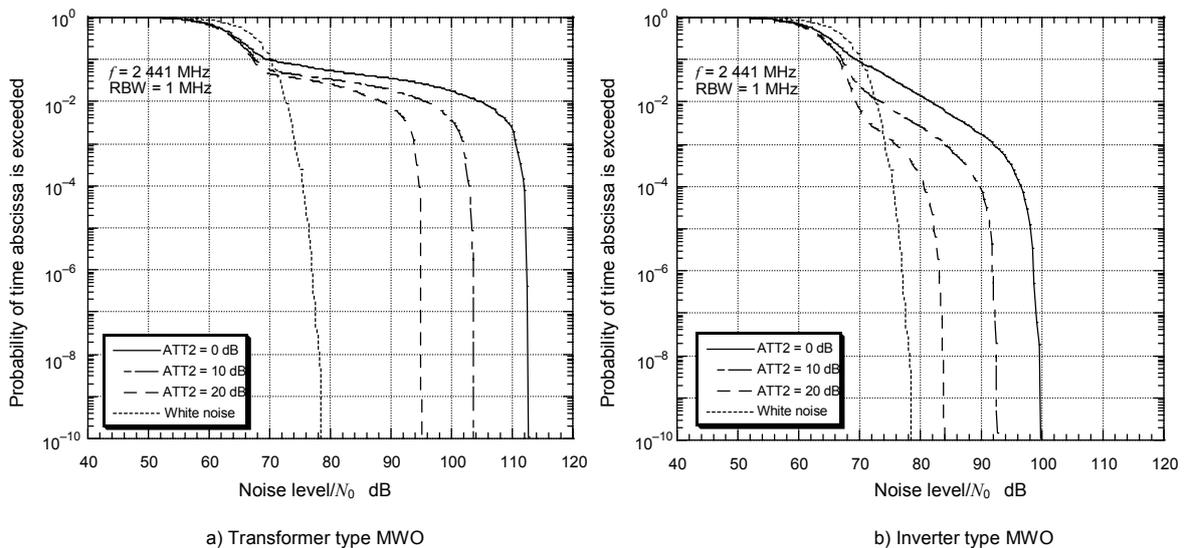
Figure 117 – APD of disturbance of actual MWO (2 441MHz)
