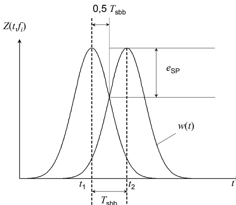
**Figure 184 – Measurement error for a single pulse**
