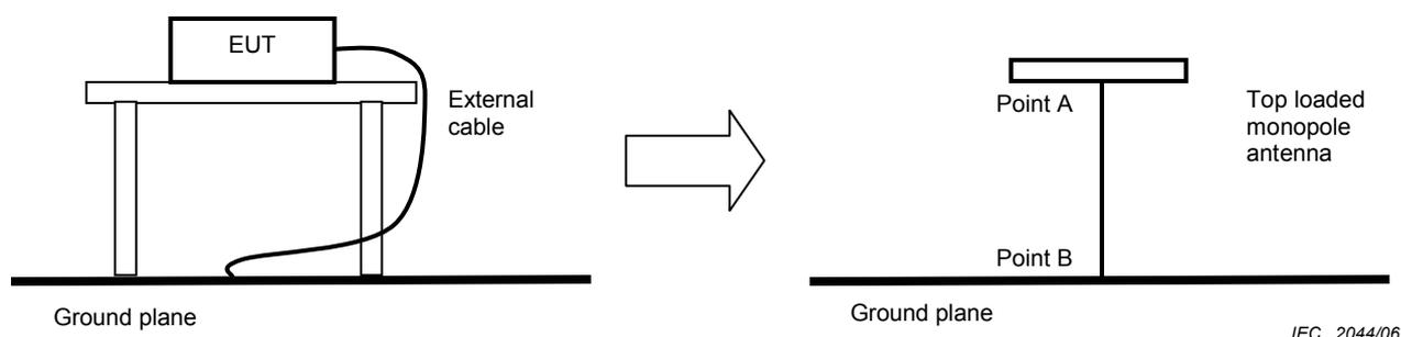
**Figure 172 – Example of a simple EUT model**
