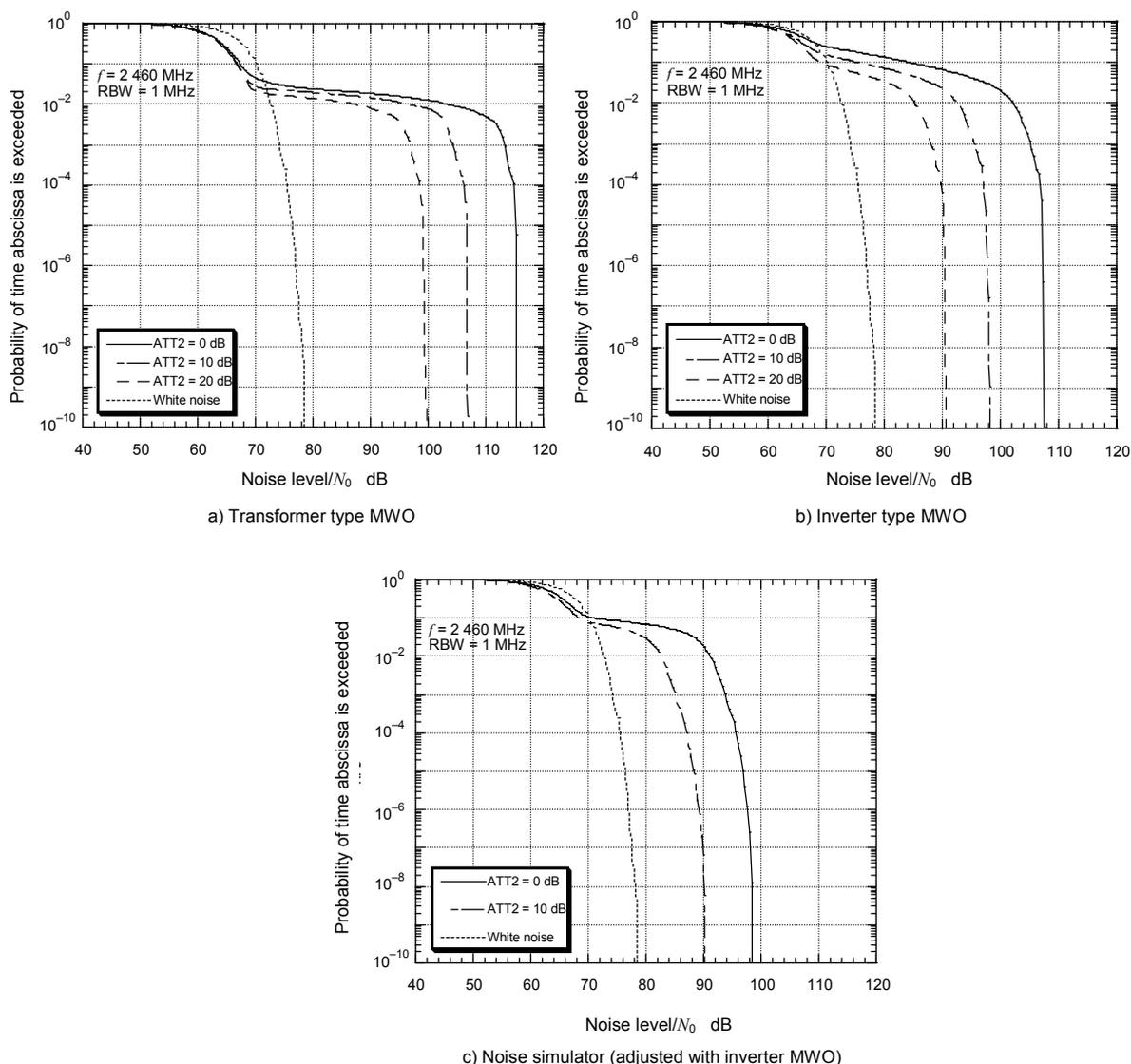
**Figure 118 – APD characteristics of disturbance (2 460 MHz)**
