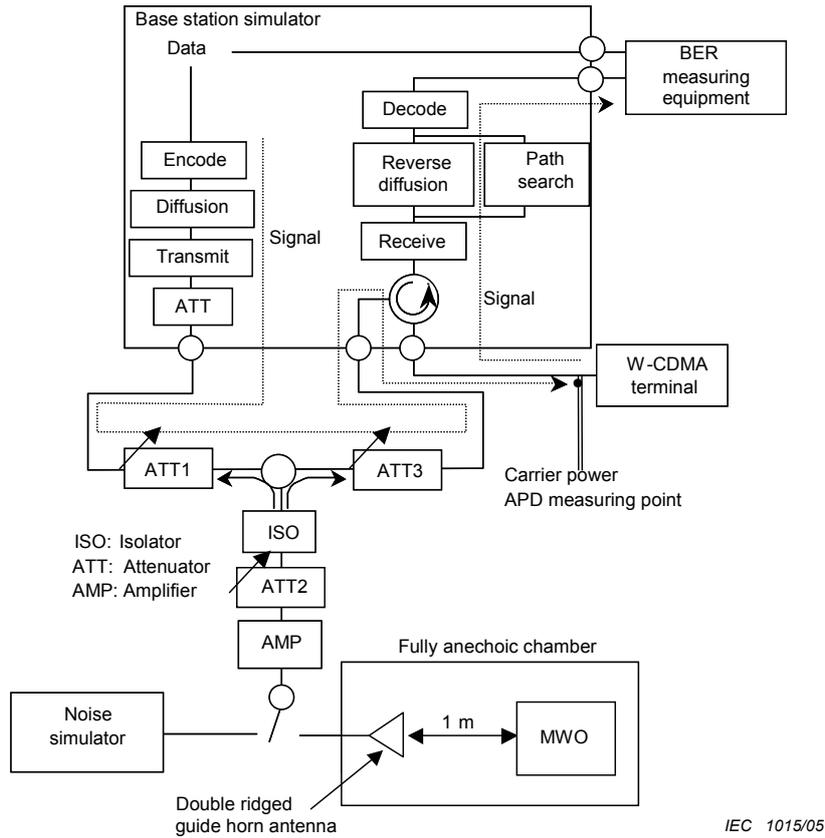
Figure 120 – Set-up for measuring the BER of W-CDMA
