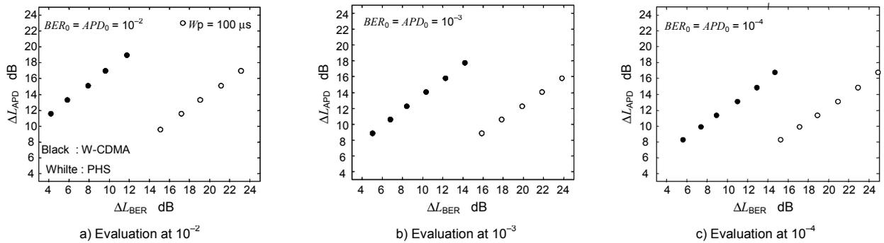
**Figure 138 – Correlation between measured  $\Delta L_{BER}$  and  $\Delta L_{APD}$**
