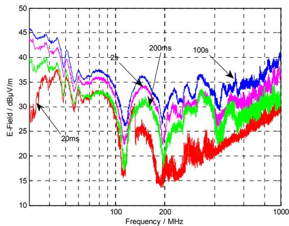
**Figure 197 – Radiated emission measurement of a motor – peak detector**
