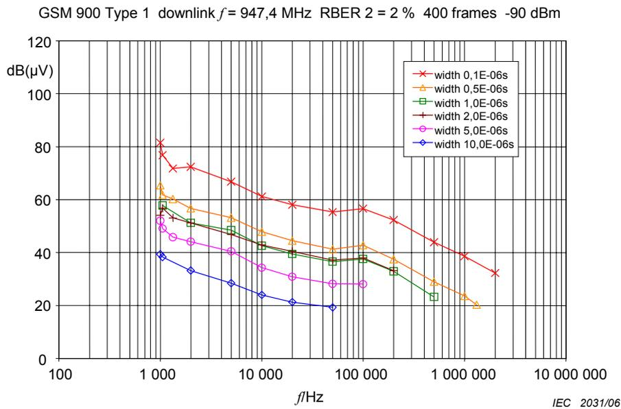
**Figure 159 – Weighting characteristics for RBER 2 of GSM**
