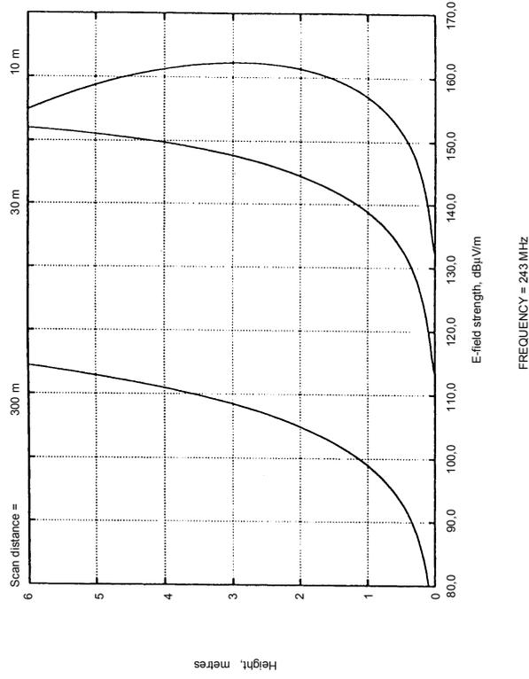
NOTE Loop dimensions  $0,05 \text{ m} \times 0,05 \text{ m}$ ; loop height  $1 \text{ m}$ ; dipole moment  $1 \text{ A}\cdot\text{m}^2$ ; horizontal distance  $10 \text{ m}$ ,  $30 \text{ m}$  and  $300 \text{ m}$ ;  $243 \text{ MHz}$ ; ground constants:  $\epsilon_r = 15$ ,  $\sigma = 4,5 \text{ mS/m}$ ; Z-X plane (Reproduced from [39]).
