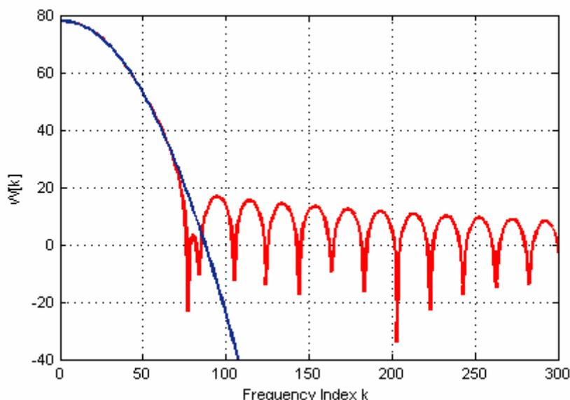
Figure 183 – Sidelobe effect due to the finite length of window
