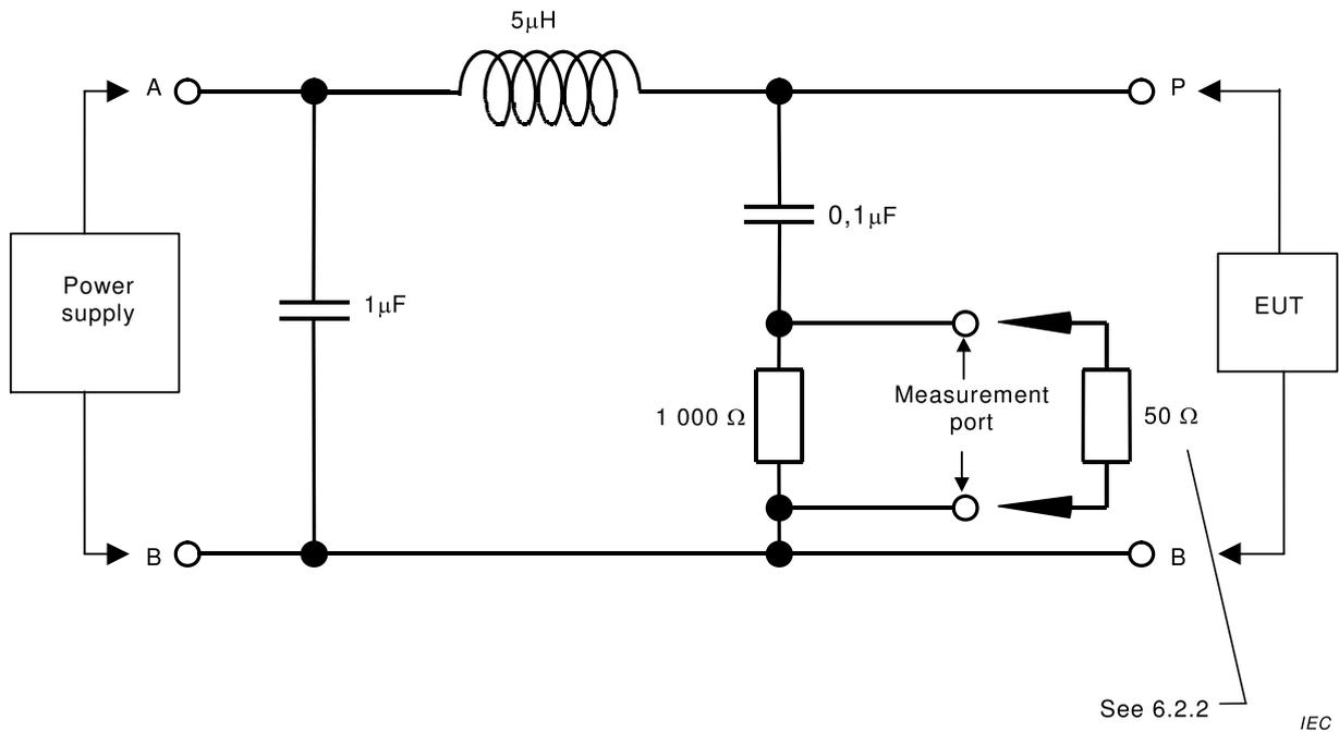
Figure E.1 – Example of 5 μH AN schematic
