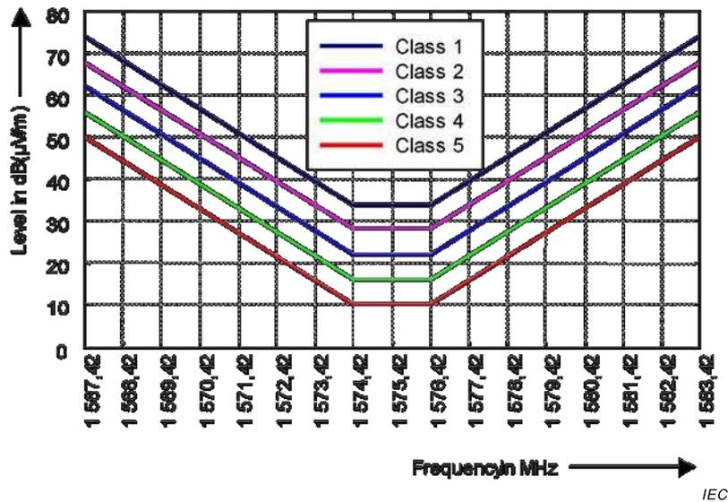
Figure 19a – GPS band 1 567,42 MHz to 1 583,42 MHz
