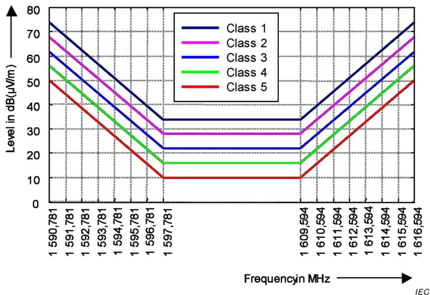
Figure 19b – GLONASS band 1 590,781 MHz to 1 616,594 MHz
