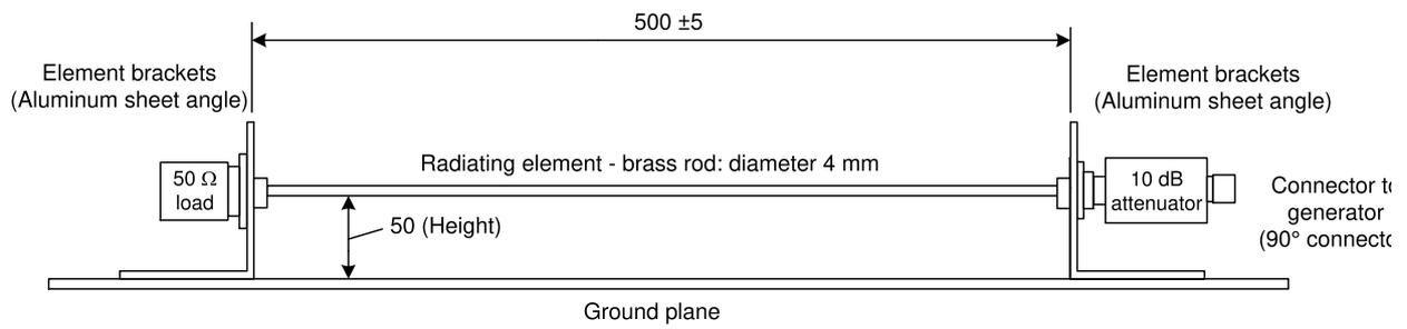
**Figure J.9 – Radiator side view 50 Ω terminations**
