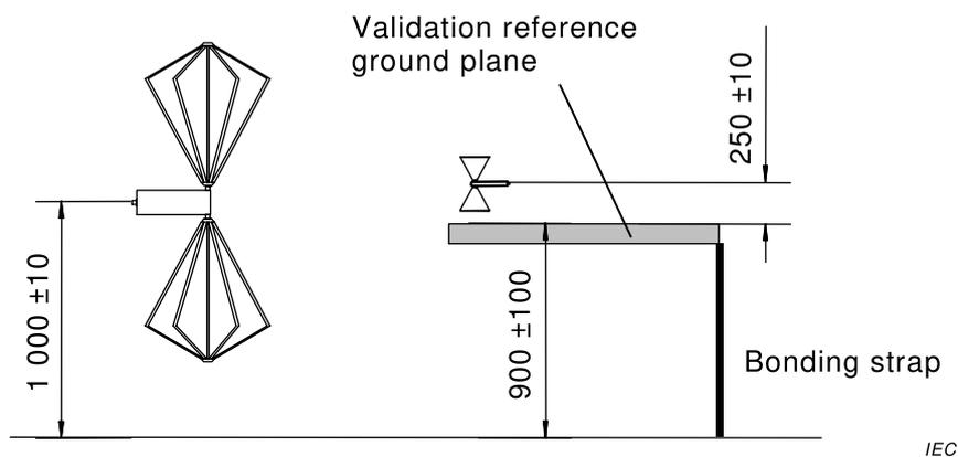
**Figure J.6 – Side view of antenna configuration for reference measurement 30 MHz and above (with the biconical antenna shown as example)**
