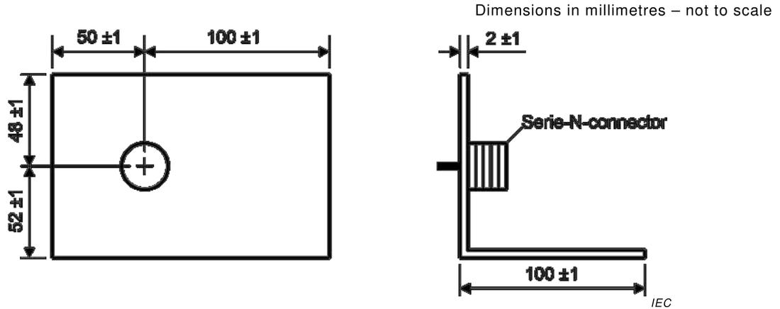
NOTE The two metallic sheet angles are mirror-inverted to each other.
