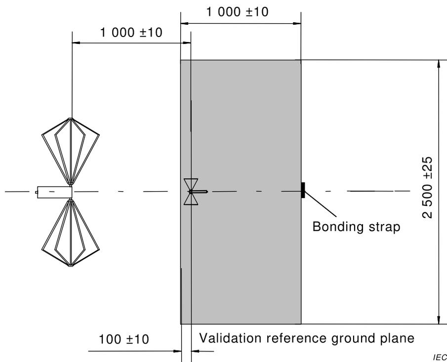
**Figure J.5 – Top view of antenna configuration for reference measurement 30 MHz and above (with the biconical antenna shown as example)**
