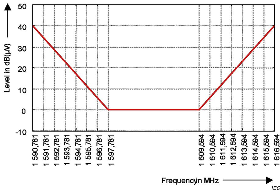
Figure 8b – GLONASS band 1 590,781 MHz to 1 616,594 MHz
