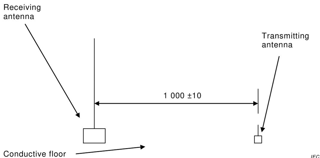
**Figure J.4 – Side view of the antenna configuration for reference measurement below 30 MHz**
