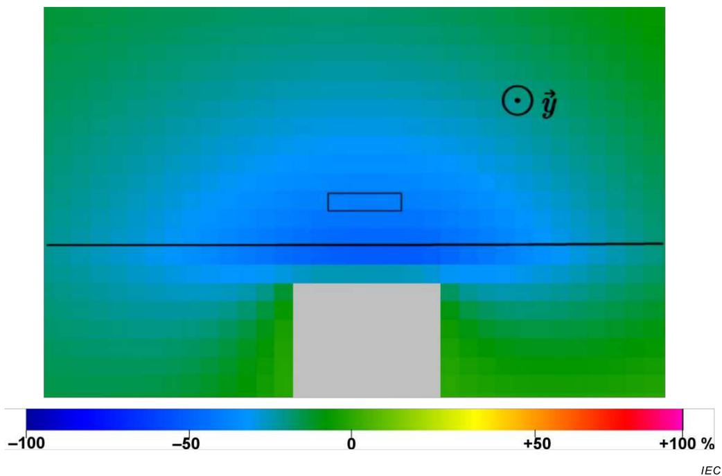
**Figure F.8 – The local y-directed momentaneous maximal electric field pattern of the condition in Figure F.3, showing the 1 mm × 1 mm voxel size and the 5 mm<sup>2</sup> integration region 2 mm above the hand underside**
