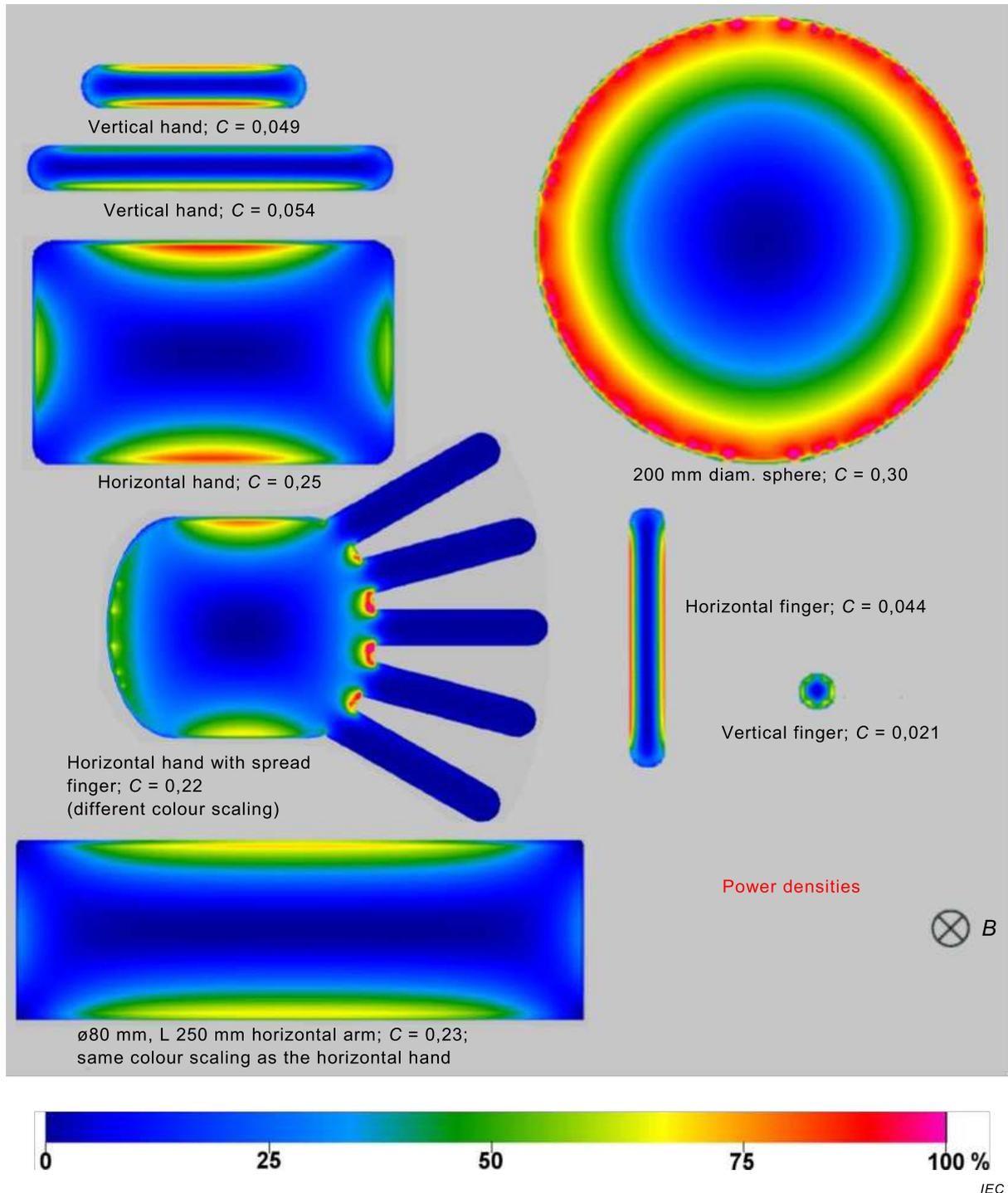
**Figure D.3 – The power density patterns in the central  $z$  plane of the reference objects, with maximal  $C$  values in m**
