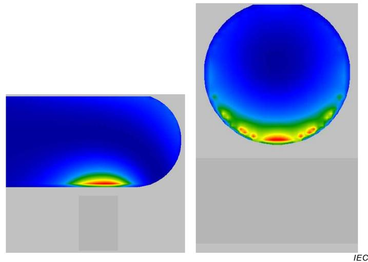
**Figure F.17 – Power density maximum pattern in the x-directed 17 mm diameter finger model**
