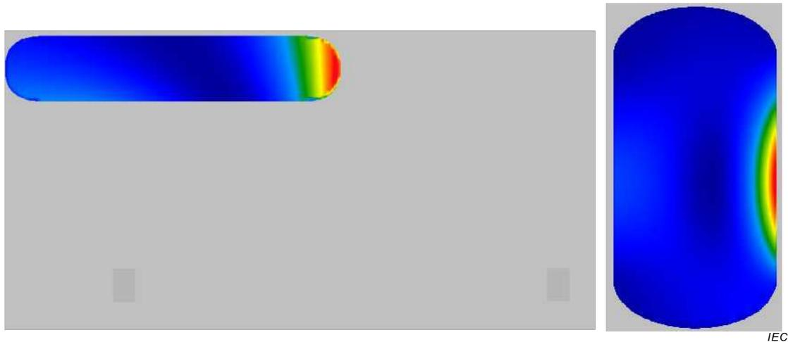
**Figure F.5 – Power density pattern in the central vertical plane and in the bottom 1 mm layer of the hand model,  $z = 50$  mm;  $a = -51$  mm**
