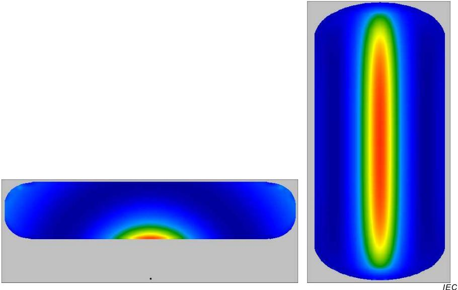
Figure E.6 – Power density in the hand model 14 mm above the wire axis
