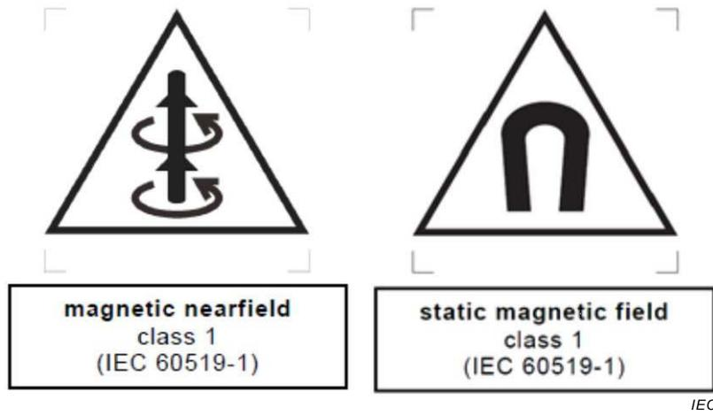
Figure 1 – Examples of warning marking
