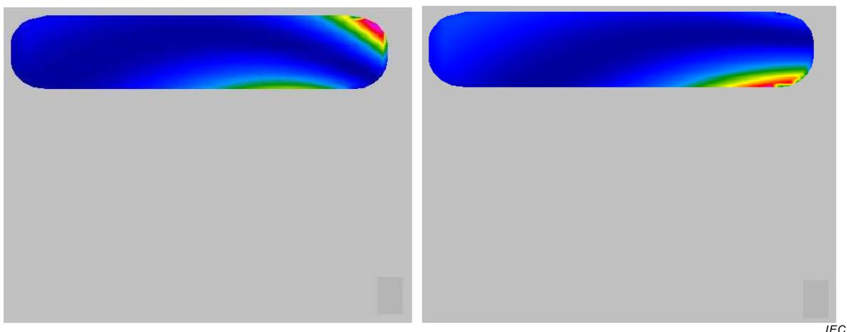
**Figure F.14 – The power density in the central vertical cross section of the hand as in the scenario in Figure F.11, but 50 mm above the coil; with no workload (left) and with permeable metallic workload (right)**
