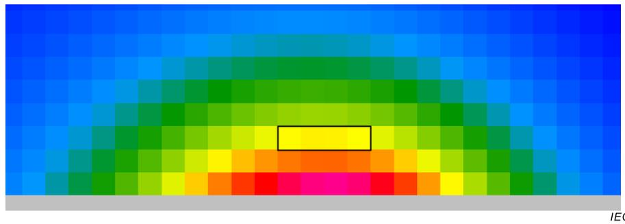
**Figure F.7 – The local power density pattern of the condition in Figure F.3, showing the 1 mm × 1 mm voxel size and the 5 mm<sup>2</sup> integration region 2 mm above the hand underside**
