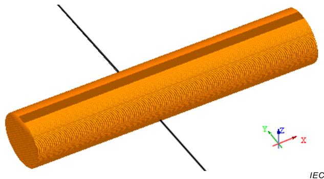
**Figure E.9 – Wrist/arm model above a long straight wire**
