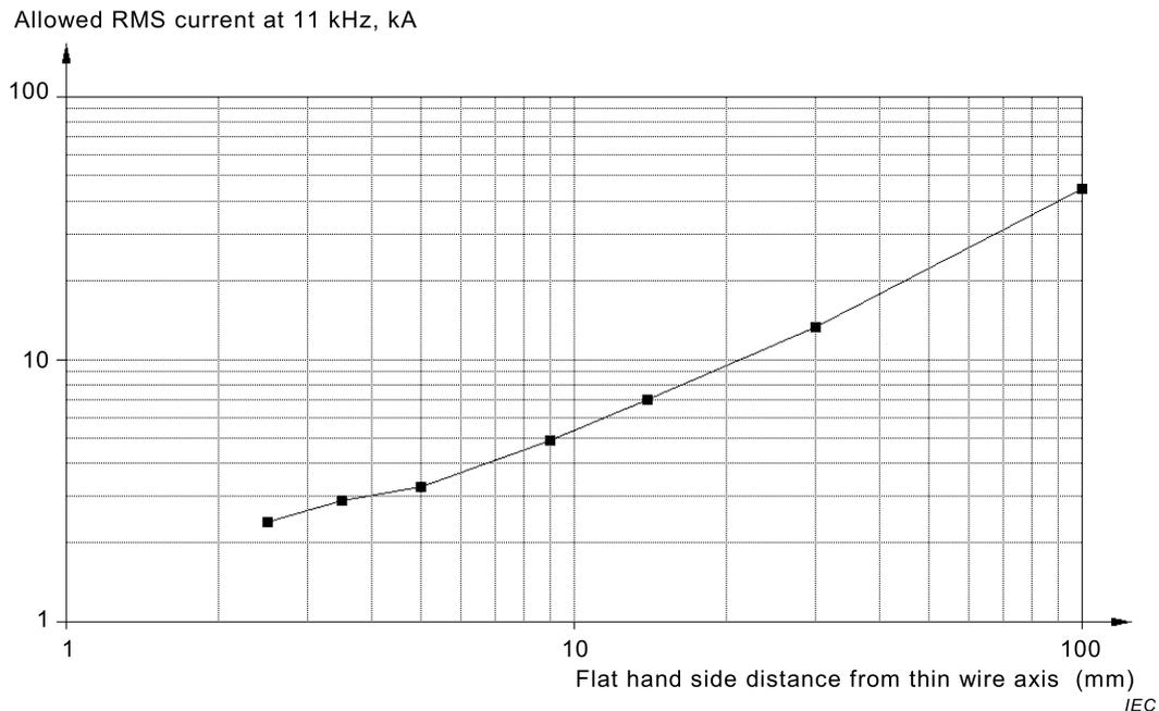
Figure G.1 – Allowed RMS current at 11 kHz, based on CGCR =  $40 \text{ Vm}^{-1}$
