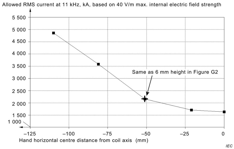
**Figure G.3 – CGCR coil currents at 11 kHz for the hand model at 6 mm above the coil with different sideways positions**
