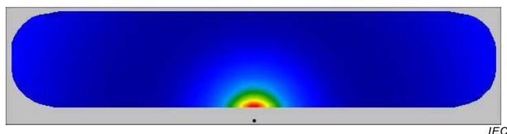
Figure E.5 – Power density in the hand model 2,5 mm above the wire axis
