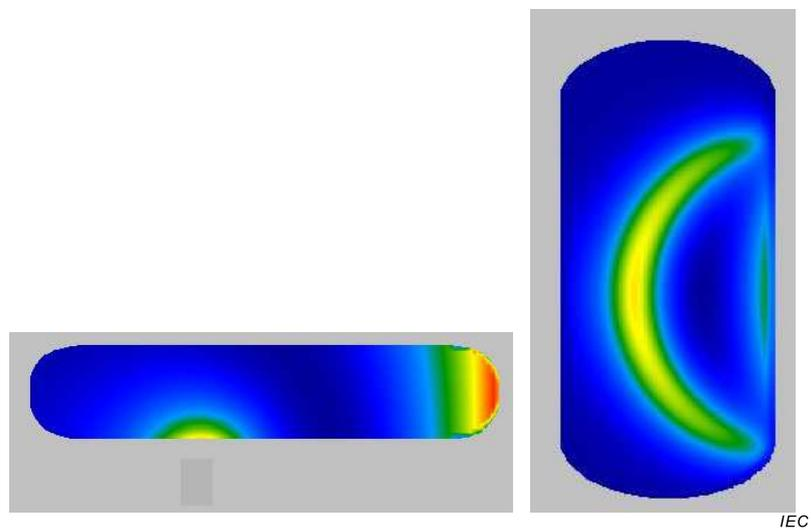
**Figure F.4 – Power density pattern in the central vertical plane and in the bottom 1 mm layer of the hand model,  $z = 4 \text{ mm}$ ;  $a = -51 \text{ mm}$**
