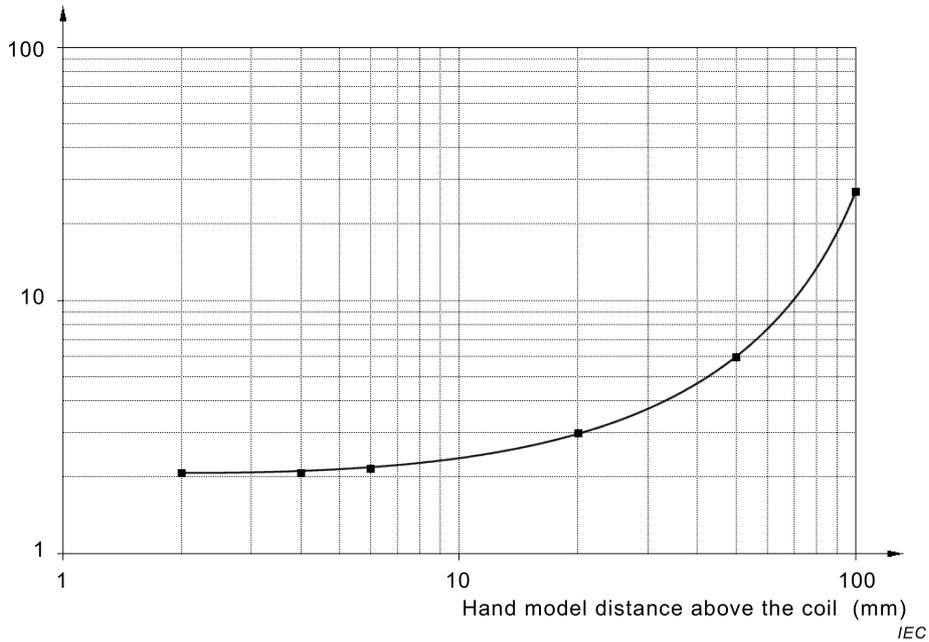
**Figure G.2 – CGCR coil currents at 11 kHz for the hand model with the side at the coil axis, at various heights above the coil**
